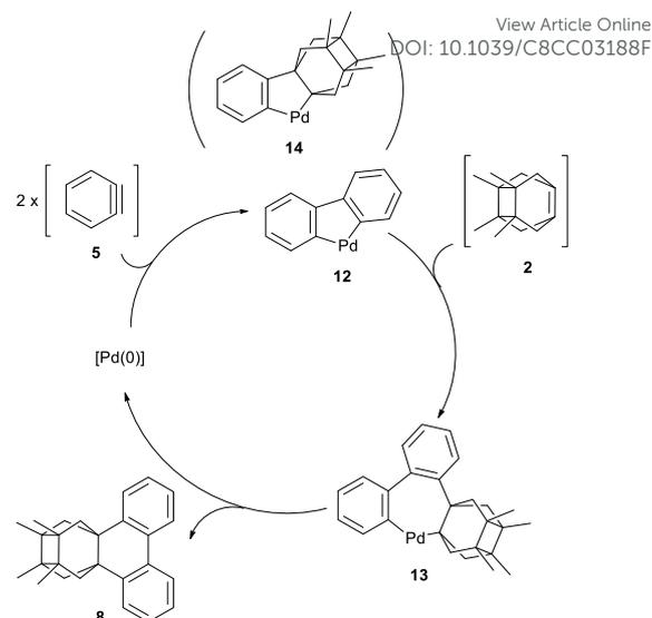
**Scheme 3.** Proposed reaction mechanism for cocyclotrimerization of pyramidalized alkene **2** and benzyne (**5**).
