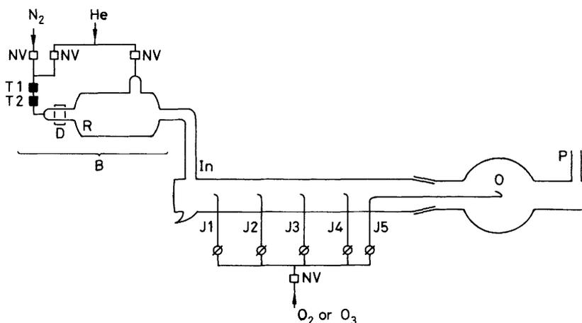
Fig. 1. Schematic diagram of the apparatus. B, discharge bypass; D, discharge cavity; In, atom inlet to flow tube; J1–J5, fixed injectors; NV, needle valve; O, observation region; P, pressure port; T1, molecular-sieve trap; T2, glass-wool trap.
