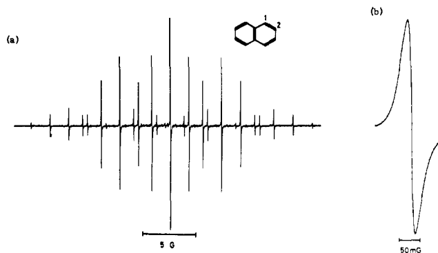
Figure 1. ESR spectra of the naphthalene radical anion in HMPA at room temperature, scan time 2 hr, modulation frequency 10 kHz, modulation amplitude 10 mG: (a) full spectrum, range 40 G, a_1 = 4.92 G, a_2 = 1.79 G; (b) an expanded spectrum of the center part, range 1 G.
