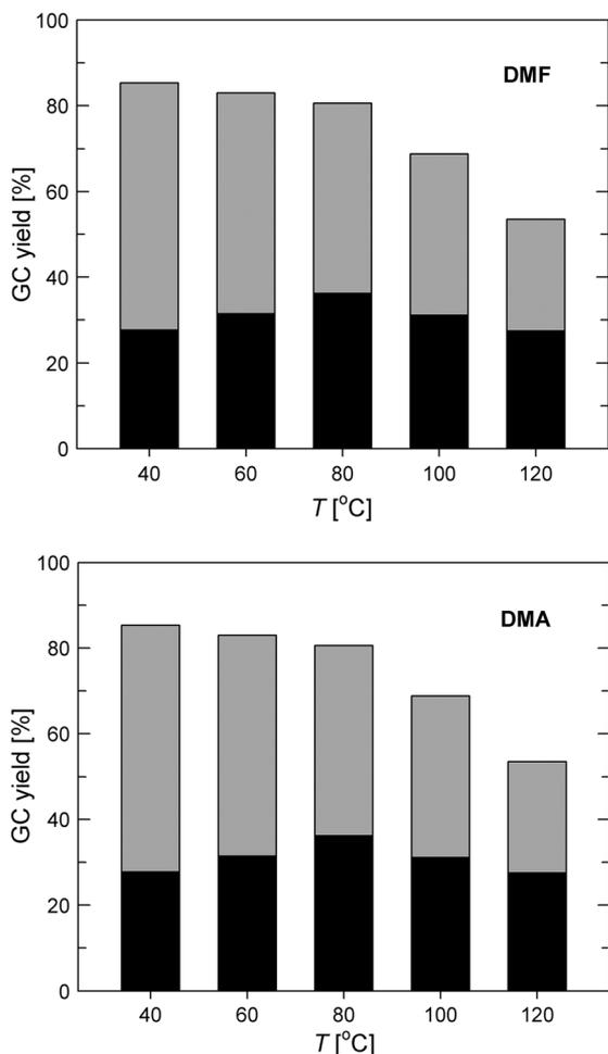
**Figure 6.** Influence of the reaction temperature on the yield of the coupling reaction. Black bars represent the yield of the coupling product **10**, gray bars that of biphenyl **11**. Conditions:  $\text{PhSnBu}_3$  (1.0 mmol), 4-bromotoluene (1.0 mmol), KF (2.0 mmol), mesitylene (1.0 mmol) and catalyst **6b** (0.5 mol% Pd), reaction in DMF or DMA (4 ml) at 80°C for 24 h.
