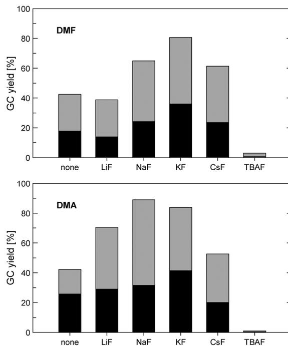
**Figure 5.** Influence of fluoride additives on the course of the coupling reaction. Black bars represent the yield of the coupling product **10**, gray bars that of biphenyl **11**. Conditions: PhSnBu<sub>3</sub> (1.0 mmol), 4-bromotoluene (1.0 mmol), additive (2.0 mmol), mesitylene (1.0 mmol; internal standard) and catalyst **6b** (0.5 mol% Pd), reaction in DMF or DMA (4 ml) at 80°C for 24 h. TBAF, [Bu<sub>4</sub>N]F·3H<sub>2</sub>O.
