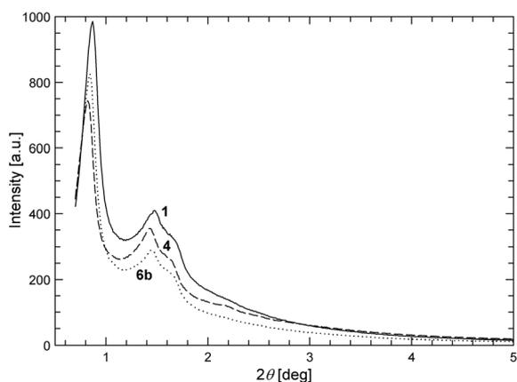
**Figure 2.** Small-angle X-ray diffraction patterns of materials **1** (solid line) and **4** (dashed line) and catalyst **6b** (dotted line).
