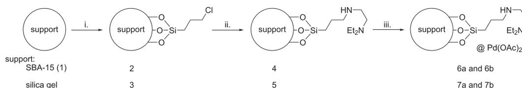
**Scheme 1.** Preparation of Pd catalysts **6** and **7**. Legend: *i*, (3-chloropropyl)triethoxysilane in toluene, refluxing (repeated twice); *ii*, treatment with  $\text{Et}_2\text{NCH}_2\text{CH}_2\text{NH}_2$  in toluene and then with ammonia in ethanol–water; *iii*,  $\text{Pd}(\text{OAc})_2$  in dichloromethane.
