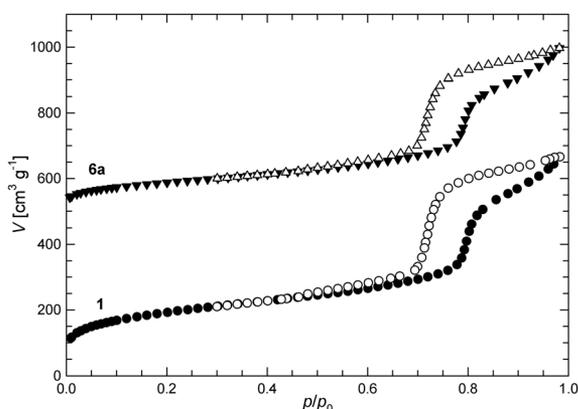
**Figure 3.** BET adsorption isotherms for the parent SBA-15 (**1**; circles) and material **6a** (triangles). Filled symbols, adsorption; empty symbols, desorption.
