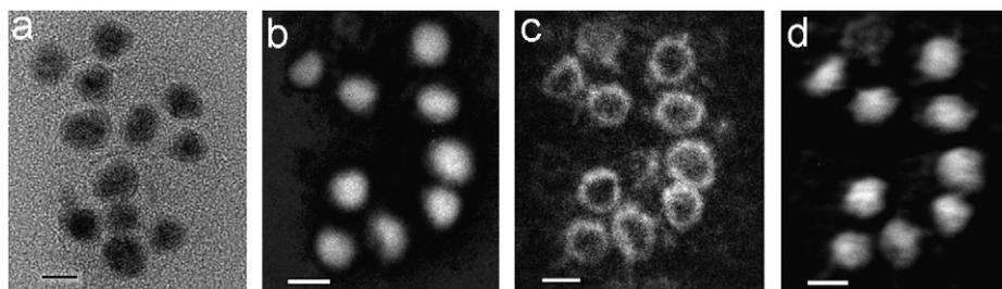
Fig. 4. TEM image of  $\text{SiO}_2$  coated Co particles (a) and EFTEM images (Co map (Co  $L_{2,3}$  edge) (b), O map (O K edge) (c), and Si map (Si  $L_{2,3}$  edge) (d)) (scale bar 10 nm).
