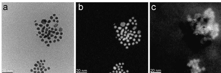
Fig. 2. Co nanoparticles coated by carbomethoxydextran and corresponding EFTEM images (Co map (Co  $L_{2,3}$  edge) (b), and O map (O K edge) (c)) (scale bar 20 nm).
