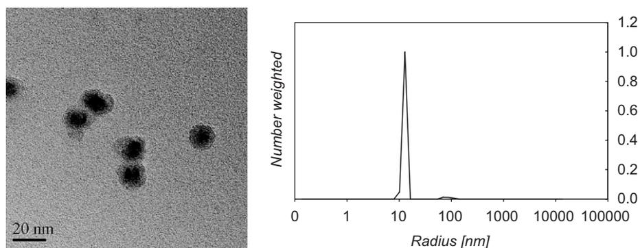
Fig. 3. TEM image of  $\text{SiO}_2$  coated Co particles (scale bar 20 nm) and dynamic light scattering (DLS).
