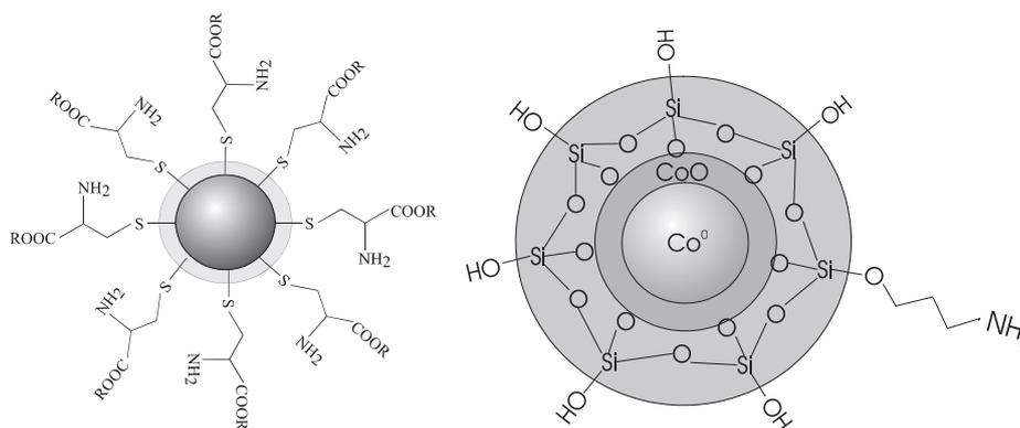
Fig. 1. Surface-modified Co nanoparticles: surface modification via a surface-active thiol group using L-cysteine ethyl ester and via a silica network exhibiting functional silanol groups.
