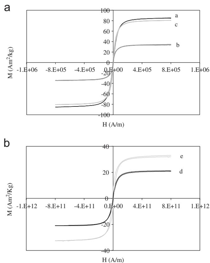
Fig. 6. Magnetization curves of *pre-stabilized* Co nanoparticles (a), individually SiO<sub>2</sub> coated Co nanoparticles (SiO<sub>2</sub> coating of Co nanoparticles stabilized by oleic acid, 50 wt% Co (b), and SiO<sub>2</sub> coating of Co nanoparticles in the absence of NH<sub>4</sub>OH, 73 wt% Co (c)) and Co nanoparticles embedded in SiO<sub>2</sub> microspheres (24 wt% Co (d)) and poly(MMA–DVB) microspheres (35 wt% Co (e)).
