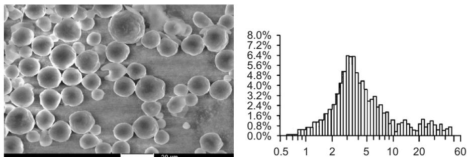
Fig. 5. SEM image of Co nanoparticles embedded in poly(MMA–DVB) microspheres (size around 15 μm) and size distribution of poly(VA–DVB) microspheres (size around 3 μm).
