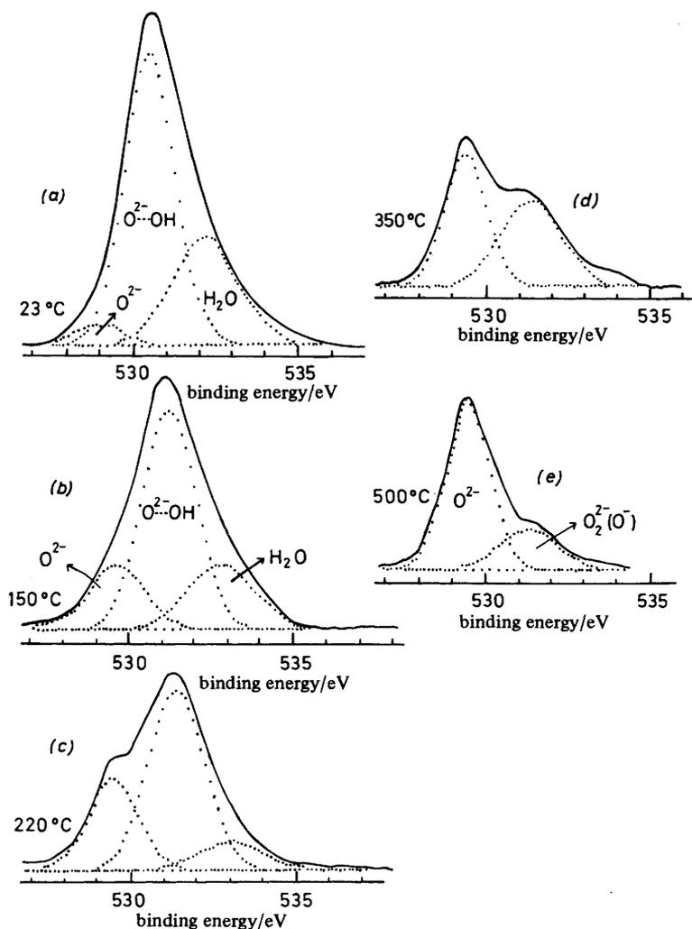
Fig. 4. O(1s) curve-fitted spectra for  $\beta\text{NiO}(\text{OH})$  and during thermal decomposition with peak assignments. (a) 296, (b) 423, (c) 493, (d) 623 and (e) 773 K.
