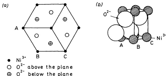
Fig. 5. Two views of  $\beta\text{NiO}(\text{OH})$  showing (a) the plane of Ni atoms and (b) the Ni and  $\text{OH} \cdots \text{O}$  layers
