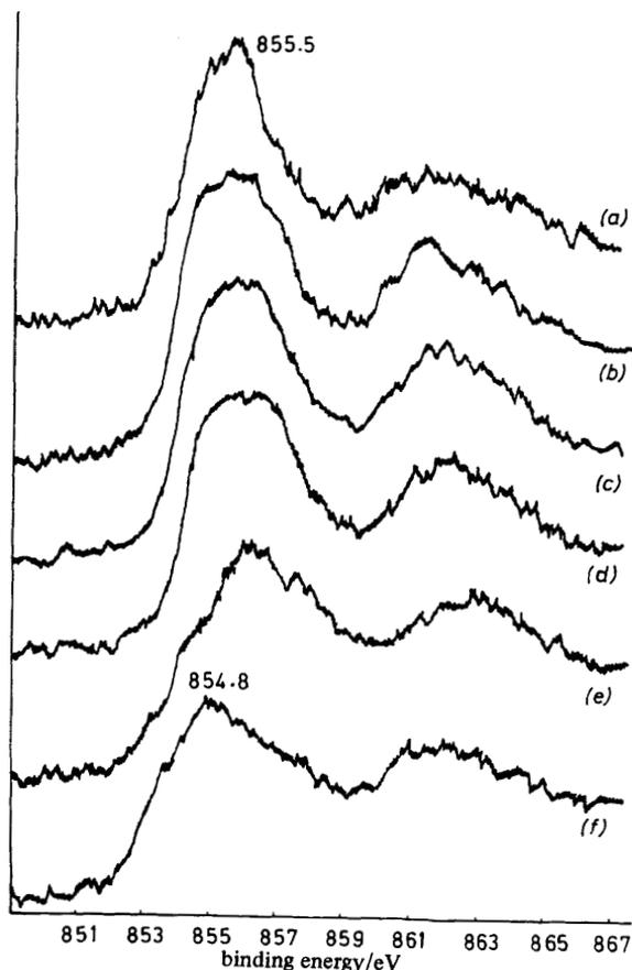
Fig. 7. Ni( $2p_{3/2}$ ) spectra corresponding to the O( $1s$ ) spectra of fig. 6.
