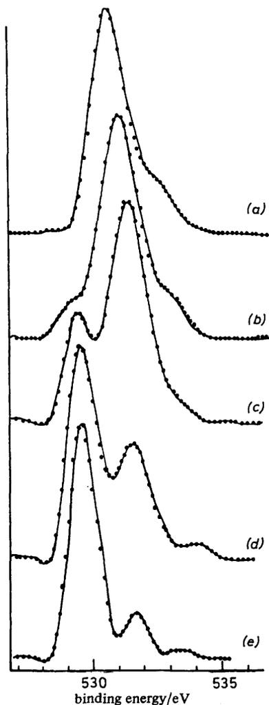
**Fig. 3.** Deconvoluted O(1s) spectra for thermal decomposition of  $\beta$ -NiO(OH); see fig. 1 above. (Scaled to same maximum.)
