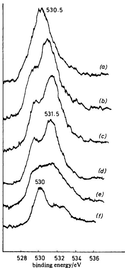
**Fig. 6.** O(1s) spectra for 'nickel peroxide' at 296 K and an ambient pressure of  $5 \times 10^{-7}$  Torr (a) and after heating (b) 423, (c) 453, (d) 493, (e) 623 and (f) 773 K.
