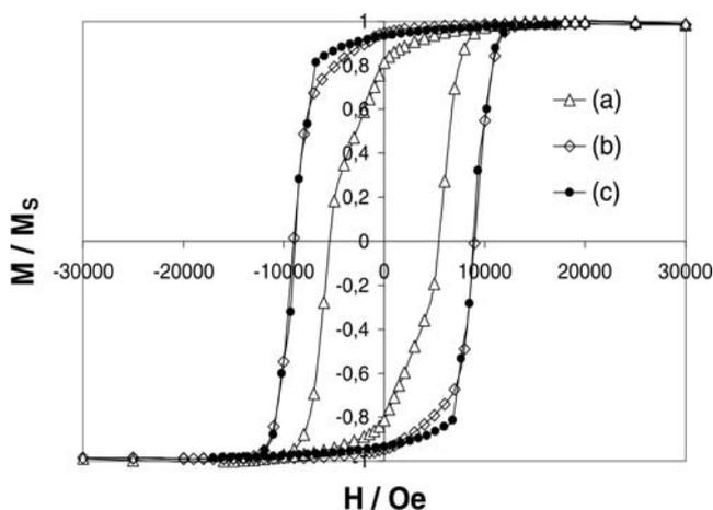
**Figure 2** Magnetization curves of cobalt nanorods ( $L_m = 100$  nm;  $d_m = 12.5$  nm), (a) deposited on a flat substrate with an external magnetic field ( $T = 300$  K); (b) frozen in toluene under an external magnetic field ( $T = 150$  K); (c) simulation of the frozen sample magnetization curve using the Stoner–Wolffarth model for an assembly of non-interacting wires.
