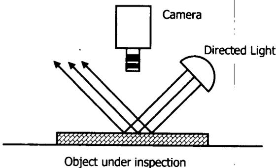
FIGURE 1. Illumination and capture set-up.
