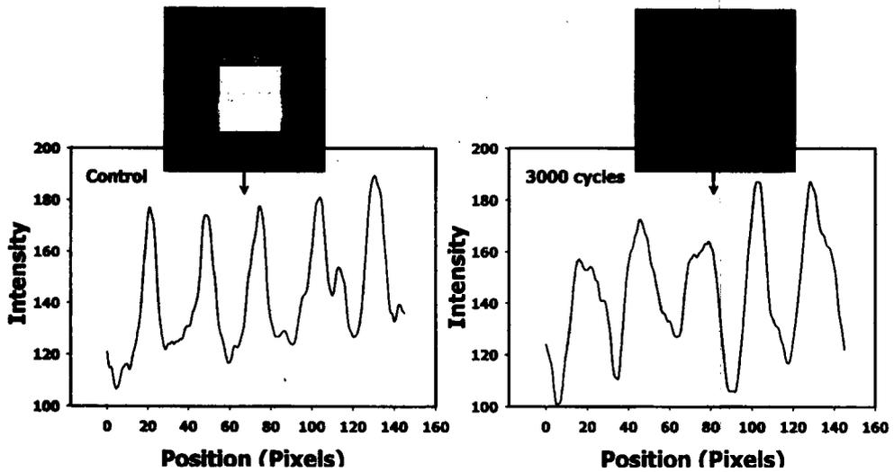
FIGURE 8. Intensity profiles for Miratec twill fabric.
