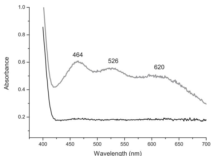
**Fig. 2.** Absorption spectra of silica gel doped with 1-vinylidene-naphthofuran **5a** before (**black**) and after (**grey**) exposure to a 6 W UV lamp (365 nm) for 60 s.
