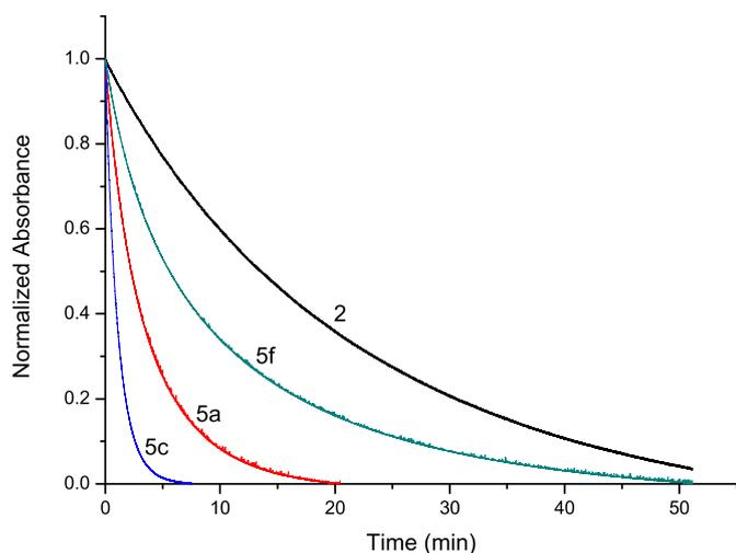
Fig. 7. Normalized thermal fading kinetics of compounds **2**, **5a**, **5c**, **5f** in THF/HCOOH, in the dark, measured at 540 nm.
