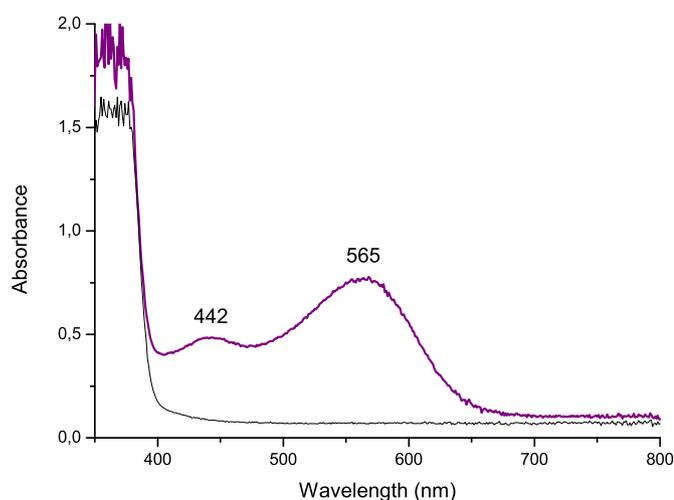
**Fig. 1.** Absorption spectra of silica gel doped with 1-vinylidene-naphthofuran **2** before (**black**) and after (**violet**) exposure to a 6 W UV lamp (365 nm) for 1 min. (For interpretation of the references to colour in this figure legend, the reader is referred to the web version of this article.)
