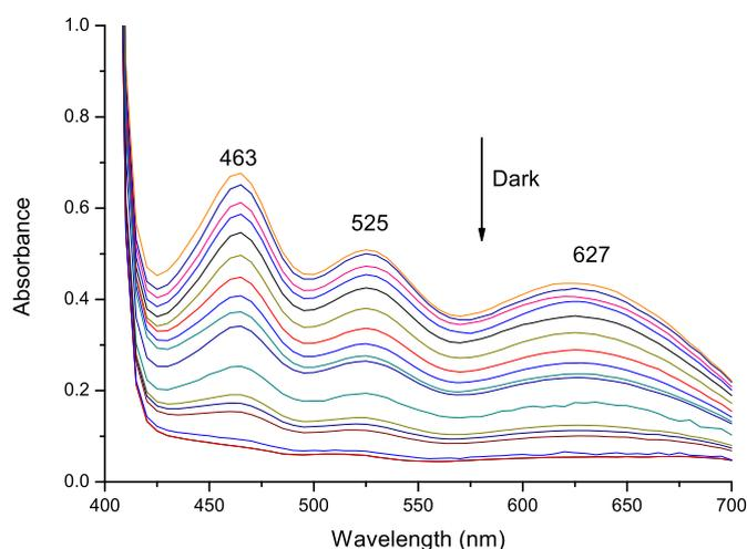
**Fig. 5.** Time evolution of the visible spectra of naphthofuran **5a** in THF/HCOOH (2/0.5) during thermal fading after UV activation with a high power laser (200 mW, 405 nm) for 60 s.
