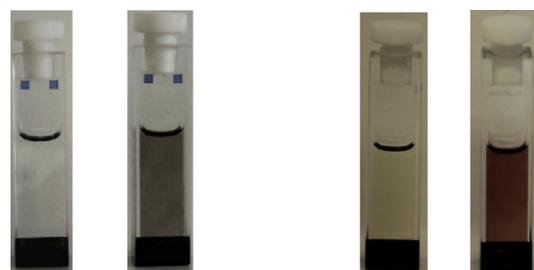
**Fig. 6.** Photographs of THF/HCOOH solutions of compounds **5a** and **5f** before and after UV irradiation (laser 200 mW, 405 nm).
