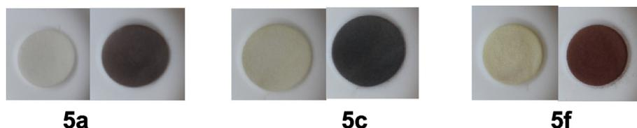
Fig. 3. Photographs of silica gel doped with compounds **5a**, **5c**, **5f** before and after UV irradiation (6 W, 365 nm) for 60 s.
