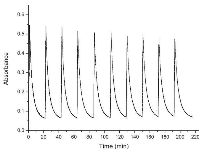
Fig. 8. UV exposure (60 s)/dark cycles of naphthofuran **5a** in THF/HCOOH at 20 °C.
