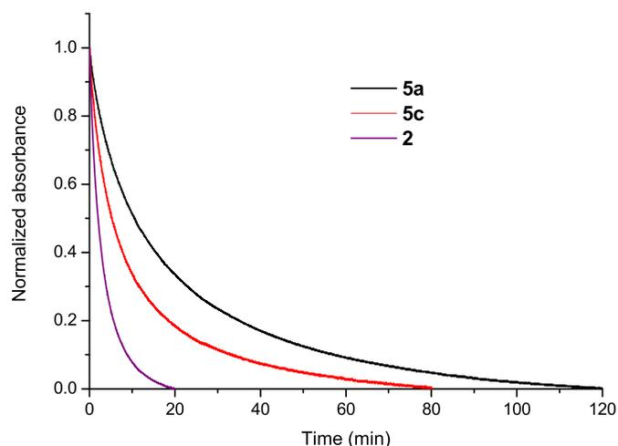
Fig. 4. Normalized thermal fading kinetics of silica gel doped with compounds **2** (violet), **5a** (black) and **5c** (red), in the dark, measured at 540 nm. (For interpretation of the references to colour in this figure legend, the reader is referred to the web version of this article.)
