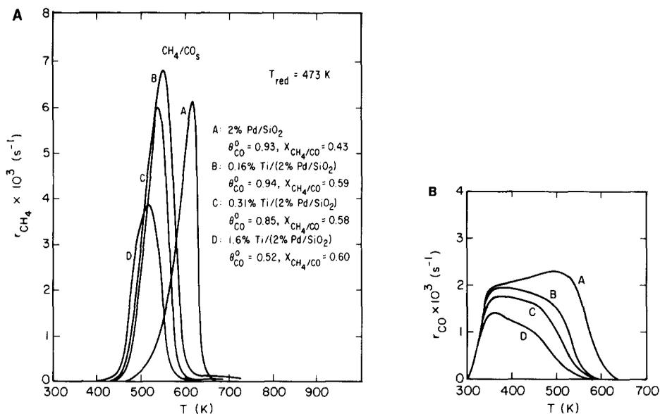
FIG. 8. Effects of titania promotion on the desorption products observed during TPSR of CO adsorbed on 2% Pd/SiO<sub>2</sub>: (A) CH<sub>4</sub>; (B) CO.
