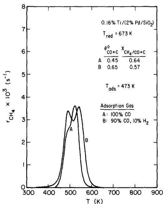
FIG. 10. Effect of the presence of H<sub>2</sub> during CO adsorption on CH<sub>4</sub> formation during TPSR of CO adsorbed on 0.16% Ti/(2% Pd/SiO<sub>2</sub>).
