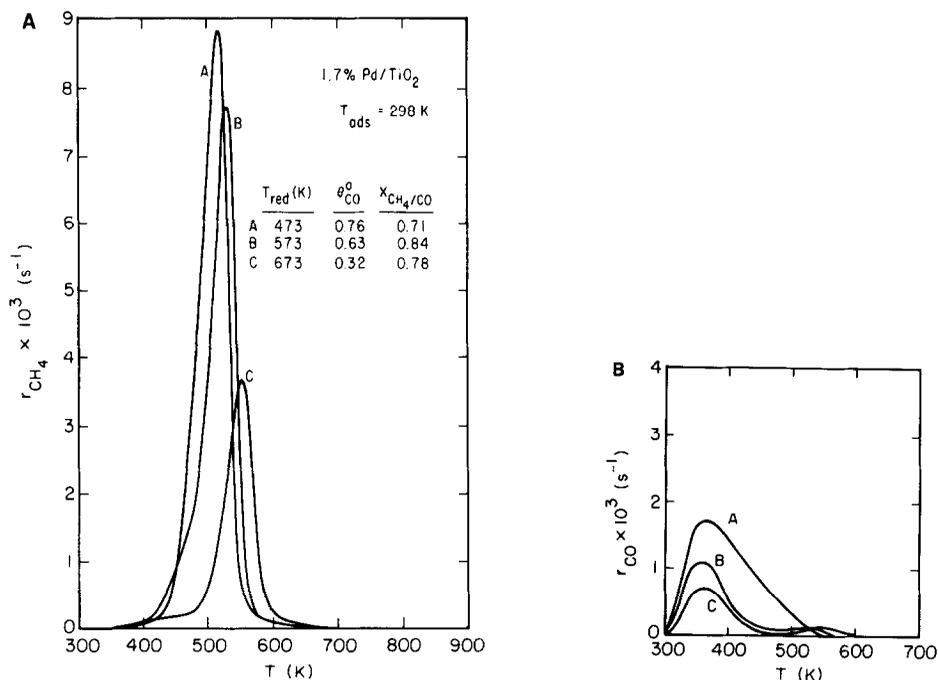
FIG. 5. Effect of reduction temperature on the products formed during TPSR of CO adsorbed on 1.7% Pd/TiO<sub>2</sub>: (A) CH<sub>4</sub>; (B) CO.
