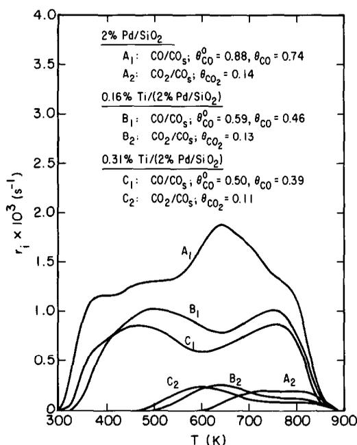
FIG. 4. Effect of titania promotion on the desorption products observed during CO TPD from 2% Pd/SiO<sub>2</sub>. Curves A<sub>1</sub>, B<sub>1</sub>, and C<sub>1</sub> represent the rate of CO desorption, while curves A<sub>2</sub>, B<sub>2</sub>, and C<sub>2</sub> represent the rate of CO<sub>2</sub> formation.
