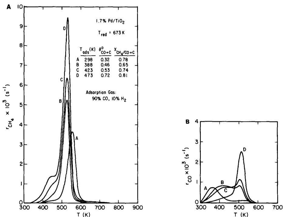
FIG. 7. Effects of the presence of H<sub>2</sub> during CO adsorption on the products formed during TPSR for 1.7% Pd/TiO<sub>2</sub>: (A) CH<sub>4</sub>; (B) CO.
