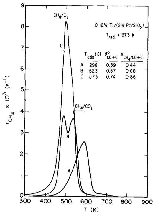
FIG. 9. Effect of CO adsorption temperature on CH<sub>4</sub> formation during TPSR of CO adsorbed on 0.16% Ti/(2% Pd/SiO<sub>2</sub>).
