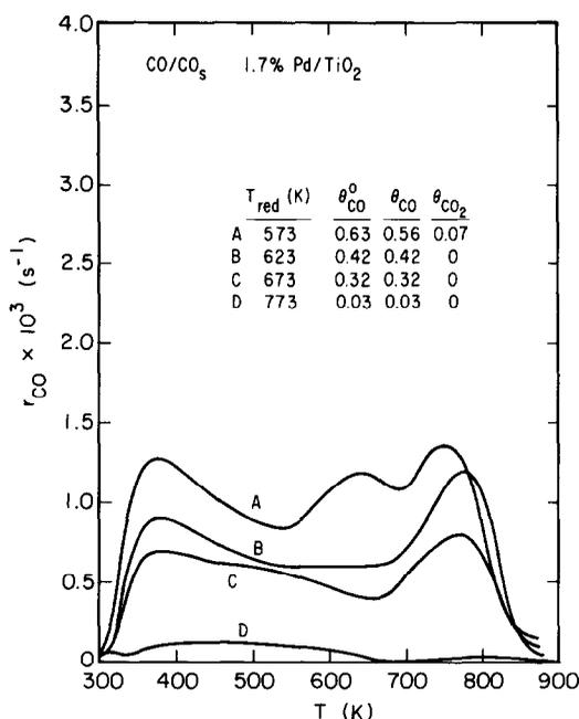
FIG. 2. Effect of reduction temperature on the CO TPD spectra for 1.7% Pd/TiO<sub>2</sub>.
