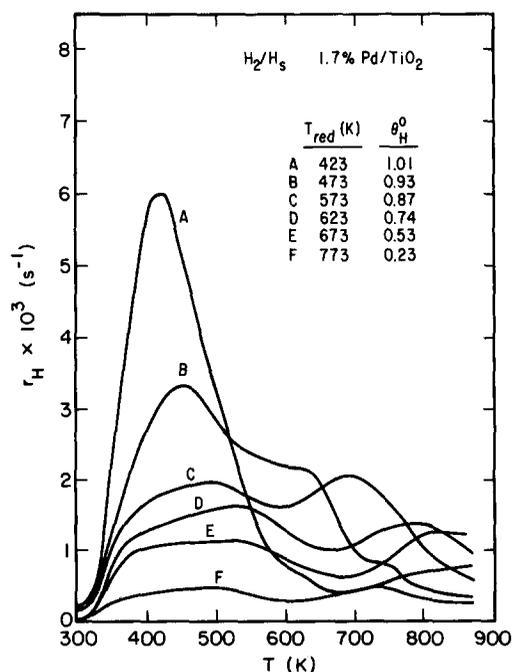
FIG. 1. Effect of reduction temperature on the H<sub>2</sub> TPD spectra for 1.7% Pd/TiO<sub>2</sub>.
