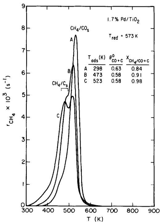
FIG. 6. Effect of CO adsorption temperature on CH<sub>4</sub> formation during TPSR of CO adsorbed on 1.7% Pd/TiO<sub>2</sub>.
