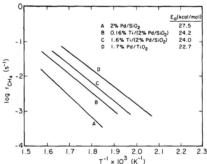
FIG. 11. Comparison of the methanation activities for Pd/SiO<sub>2</sub>, Pd/TiO<sub>2</sub>, and titania-promoted Pd/SiO<sub>2</sub>:  $P = 1$  atm,  $H_2/CO = 3/1$ .
