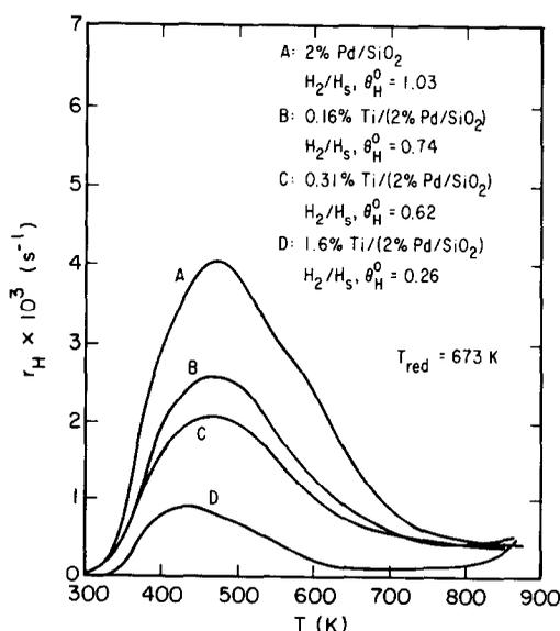
FIG. 3. Effect of titania promotion on the H<sub>2</sub> TPD spectra for 2% Pd/SiO<sub>2</sub>.
