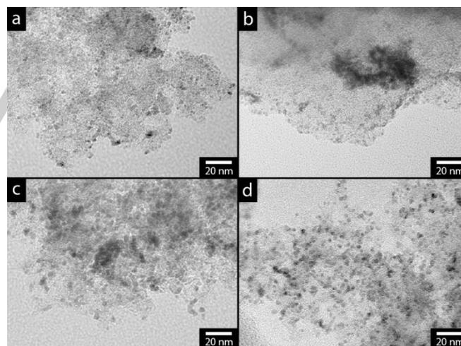
**Figure 1.** TEM images of rhodium on carbon matrix (a), rhodium on carbon matrix after drying in vacuo (b), rhodium on carbon (c) and rhodium on activated charcoal (d).
