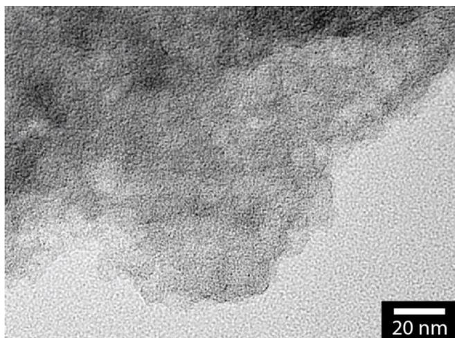
**Figure 2.** TEM image of rhodium on carbon matrix after reaction.
