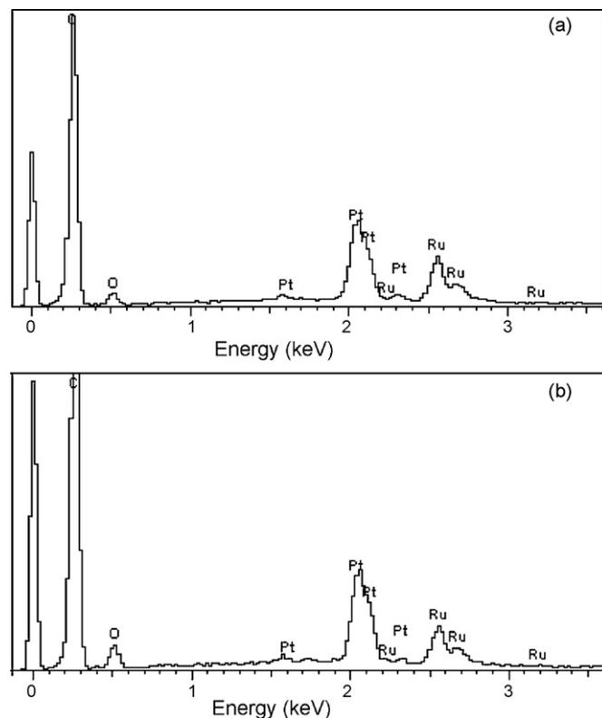
Fig. 3. EDX spectra of PtRu/CNTs (a) and PtRu/C catalysts (b).
