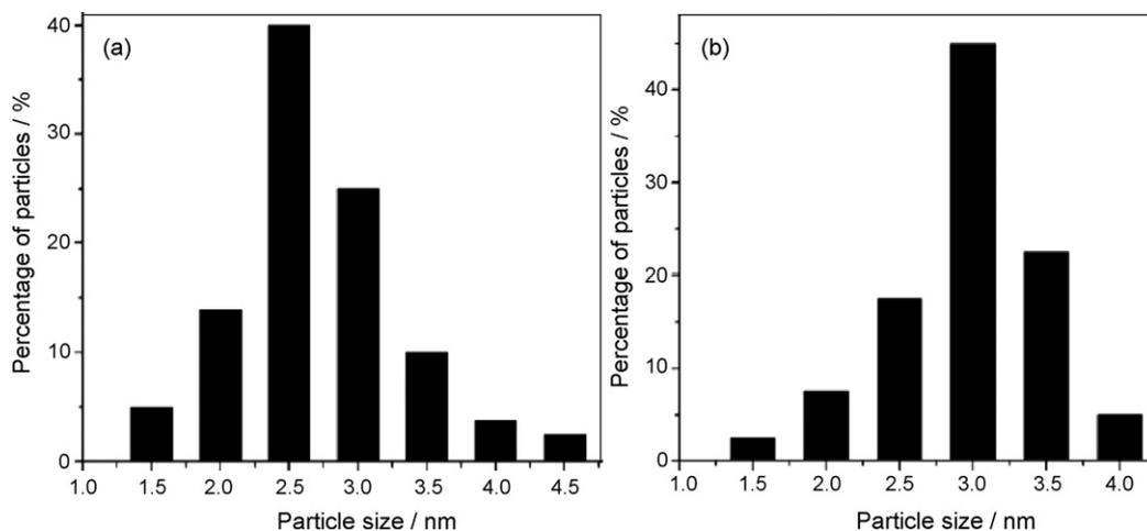
Fig. 2. Particle size distributions for PtRu nanoparticles supported on multiwalled CNTs (a) and Vulcan XC-72 carbon (b).
