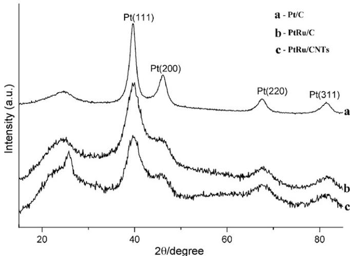
Fig. 4. XRD patterns of the catalysts prepared by modified impregnation method.
