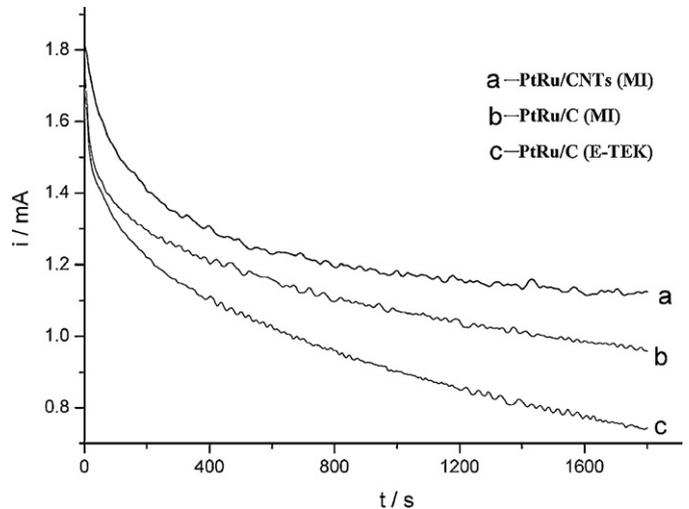
Fig. 6. Current vs. time plots measured by the CA method in 1 M CH<sub>3</sub>OH + 0.5 M H<sub>2</sub>SO<sub>4</sub> solutions at 0.5 V (vs. Ag/AgCl) at room temperature.
