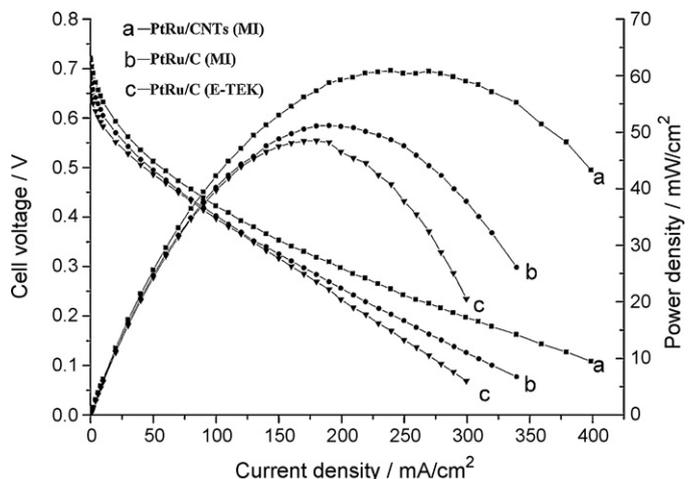
Fig. 7. Single cell performance using different PtRu catalysts at the anode at 80 °C.
