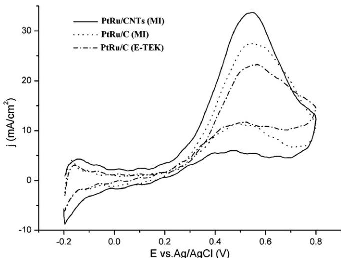
Fig. 5. Cyclic voltammograms recorded at 20 mV/s in 1 M CH<sub>3</sub>OH + 0.5 M H<sub>2</sub>SO<sub>4</sub> solutions at room temperature.
