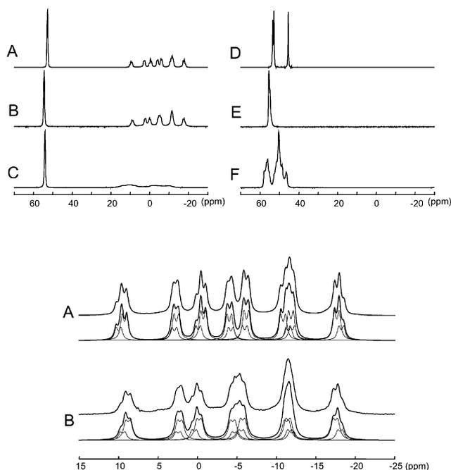
**Fig. 5**  $^{31}\text{P}\{^1\text{H}\}$  solid state CPMAS NMR spectra of mononuclear complexes  $[\text{Cu}(\text{PPh}_3)_2\text{L}]$  **6b** (A), **6a** (B), **6c** (C) and polynuclear complexes  $[\text{Cu}_n\text{L}_n]$  **7a** ( $n = 3$ ) (D), **7b** (E), **7c** (F) (top). Expansion of the experimental and simulated  $J$ -multiplet patterns of the mononuclear samples (A) and (B) (bottom).
