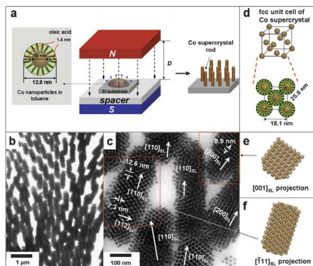
**Fig. 1** (a) Schematic of Co supercrystal formation; (b) low and (c) high magnification TEM images; (d) unit cell structure; (e)  $[001]_{\text{SL}}$  and (f)  $[111]_{\text{SL}}$  projections of fcc-structured supercrystals.
