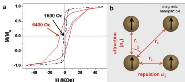
**Fig. 4** (a) Enhanced magnetism of Co supercrystal rods (red solid line) compared to that of randomly aggregated nanoparticles (black dashed line). (b) Schematic of magnetic dipole interaction between nanoparticles.
