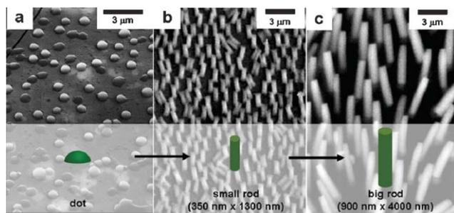
**Fig. 2** Magnetic field and concentration effects on supercrystal formation. (a) Supercrystal dots obtained in the absence of external magnetic field. (b) and (c): Supercrystal rods obtained by evaporation of 10 mM (b) and 100 mM (c) Co nanoparticle solutions.
