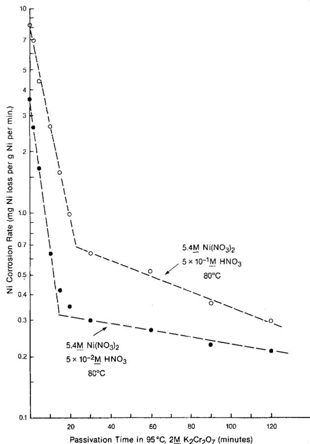
Fig. 2. Porous Ni corrosion rates in  $\text{Ni}(\text{NO}_3)_2$  solution
