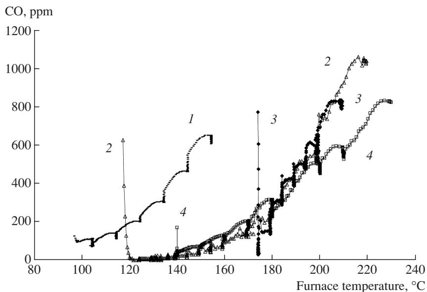
**Fig. 5.** Residual CO concentration in selective CO oxidation on (2–4) 0.1% Ru/Al<sub>2</sub>O<sub>3</sub> low-percentage catalysts as compared to (1) 1% Ru/Al<sub>2</sub>O<sub>3</sub> in the catalyst surface ignition regime during the stepwise cooling of the surface. The feed composition is the same as in Fig. 1. The gas flow rate is 91 l (g Cat)<sup>-1</sup> h<sup>-1</sup>.
