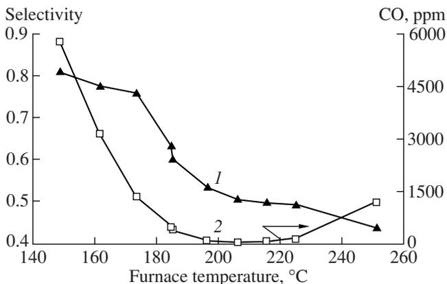
**Fig. 3.** Temperature dependence of the reaction selectivity for CO oxidation in an isothermal reactor on the 0.1% Ru/Al<sub>2</sub>O<sub>3</sub> catalyst: (1) oxygen consumption selectivity and (2) residual CO concentration. The feed composition is the same as in Fig. 1. The gas flow rate is 90 l (g Cat)<sup>-1</sup> h<sup>-1</sup>.
