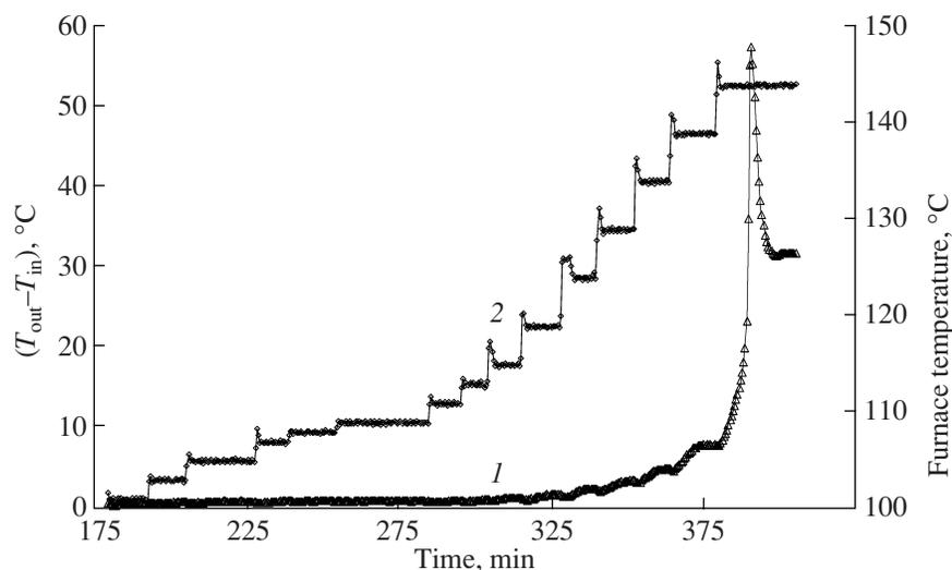
**Fig. 2.** Catalyst bed heating dynamics in selective CO oxidation on the 1% Ru/Al<sub>2</sub>O<sub>3</sub> catalyst: (1) difference between the gas temperatures at the bed exit and entrance and (2) furnace temperature. The process conditions are the same as in Fig. 1.
