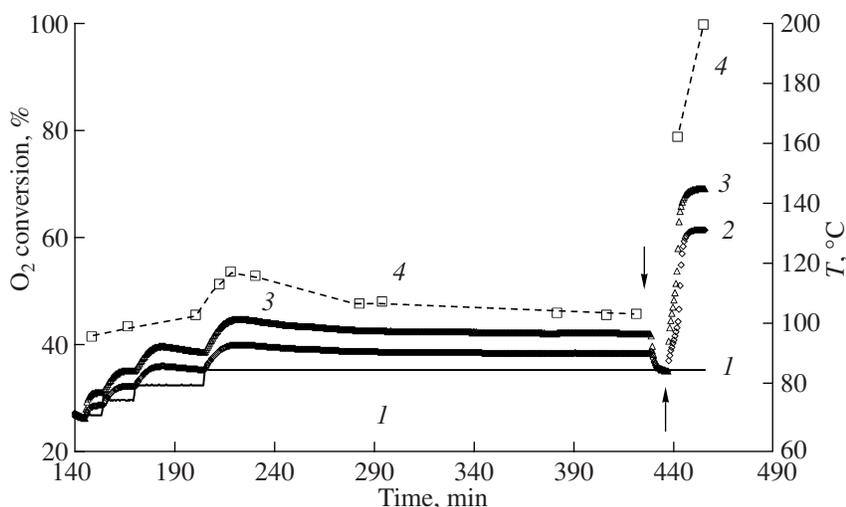
**Fig. 8.** H<sub>2</sub> oxidation on the 1% Ru/Al<sub>2</sub>O<sub>3</sub> catalyst. The arrows point to the instants H<sub>2</sub> is replaced with the reaction mixture or vice versa. (1) Furnace temperature, (2) bed entrance temperature, (3) bed exit temperature, and (4) O<sub>2</sub> conversion. Feed composition (vol %): O<sub>2</sub>, 0.98; H<sub>2</sub>, 60; N<sub>2</sub>, balance. The gas flow rate is 54 l (g Cat)<sup>-1</sup> h<sup>-1</sup>.
