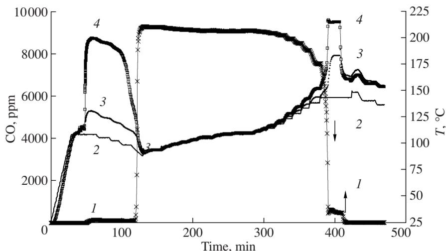
**Fig. 9.** Selective CO oxidation on the 1% Ru/Al<sub>2</sub>O<sub>3</sub> catalyst: complete record of the experimental data presented in part in Fig. 1. In the 48th minute, H<sub>2</sub> is replaced with the reaction mixture. Between the 48th and the 407th minutes, the gas flow rate is 87 l (g Cat)<sup>-1</sup> h<sup>-1</sup>; later, 17.5 l (g Cat)<sup>-1</sup> h<sup>-1</sup>. (1) Residual CO concentration, (2) furnace temperature, (3) bed entrance temperature, and (4) bed exit temperature.
