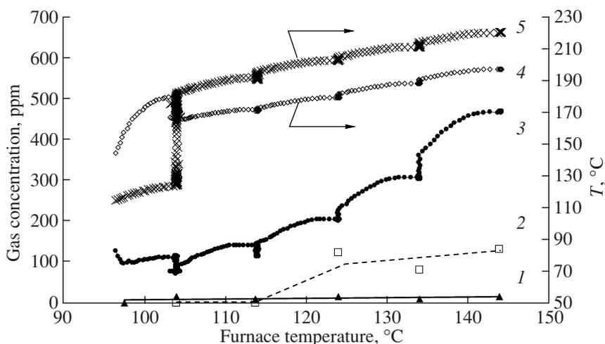
**Fig. 4.** Selective CO oxidation on the 1% Ru/Al<sub>2</sub>O<sub>3</sub> catalyst in the catalyst surface ignition regime during the stepwise cooling of the furnace: (1–3) outlet O<sub>2</sub>, CH<sub>4</sub>, and CO concentrations, respectively; (4, 5) gas temperatures at the bed exit and entrance, respectively. The feed composition is the same as in Fig. 1. The gas flow rate is 91 l (g Cat)<sup>-1</sup> h<sup>-1</sup>.
