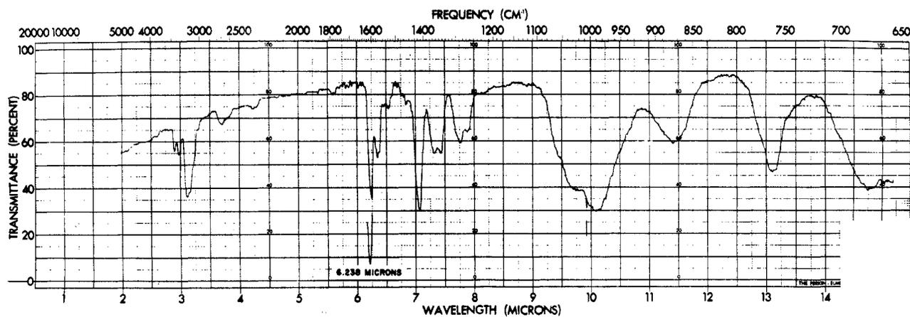
Figure 1. Infrared spectrum of condensed  $\text{Cl}_2\text{BNH}_2$  at  $-196^\circ$ .
