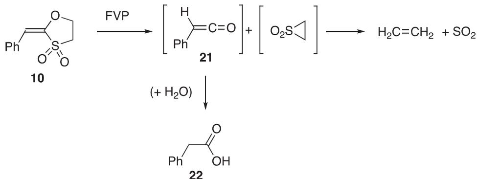
**Scheme 8.** FVP behavior of unsaturated sulfone **10**.
