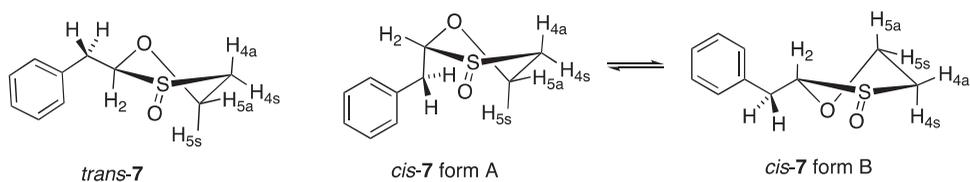
**Figure 3.** Solution conformations of *trans* and *cis*-**7** with protons labelled as *syn* (s) or *anti* (a) to the sulfoxide oxygen.
