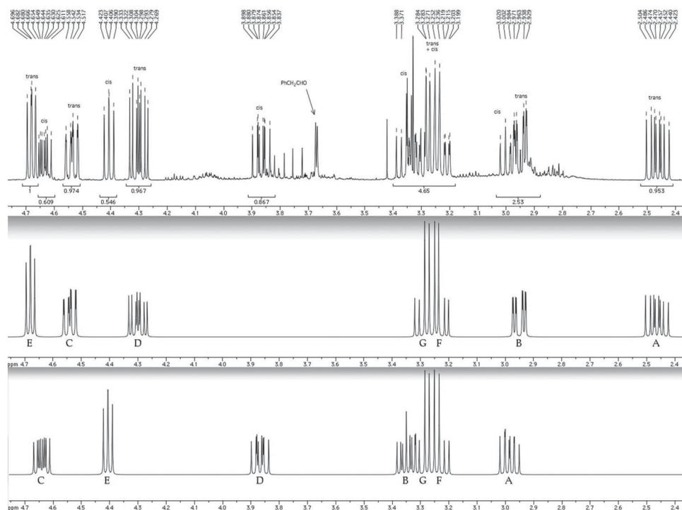
**Figure 1.** Aliphatic region of the  $^1\text{H}$  NMR spectrum of **7** showing (top) experimental spectrum for mixture of *cis* and *trans*-isomers, (middle) simulation for *trans*-**7**, and (bottom) simulation for *cis*-**7**, both using values given in Table 1.
