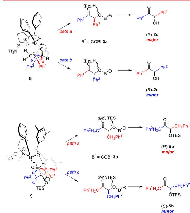
**Figure 1. Pretransition state models for enantioselective acyloin rearrangements of  $\alpha$ -hydroxy aldehyde **1c** catalyzed by **3a** and  $\alpha$ -siloxy aldehyde **4b** catalyzed by **3b**.**
