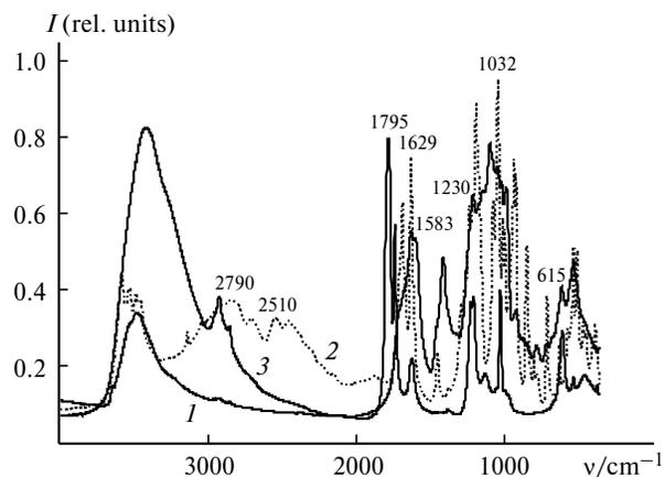
**Fig. 3.** IR spectra of the TNIC (1), PEP (2) and the product of their reaction (3). Initial concentrations of the PEP and TNIC solutions are  $1 \cdot 10^{-2} \text{ mol L}^{-1}$ .
