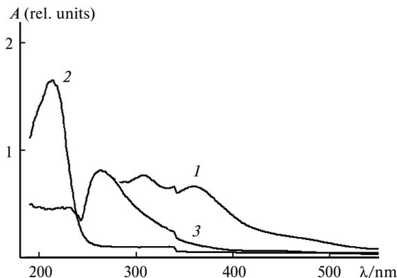
**Fig. 2.** Electronic absorption spectra of TNIC (1), PEP (2), and the product of their reaction (3). PEP concentration is  $1.05 \cdot 10^{-4} \text{ mol L}^{-1}$ ; TNIC concentration is  $1.07 \cdot 10^{-2} \text{ mol L}^{-1}$ .
