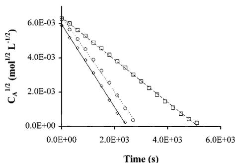
**FIGURE 2. Fit of the ethylene conversion data obtained with photocatalysis at 30 °C (□), 70 °C (○), and 107 °C (◇) with an unplatinized  $\text{TiO}_2/\text{ZrO}_2$  thin-film catalyst to a 1/2 order kinetic model.**
