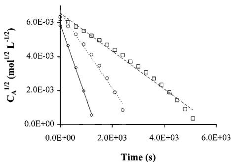
**FIGURE 3. Fit of the ethylene conversion data obtained with photocatalysis at 30 °C (□), 70 °C (○), and 107 °C (◇) with a platinized  $\text{TiO}_2/\text{ZrO}_2$  thin-film catalyst to a 1/2 order kinetic model.**
