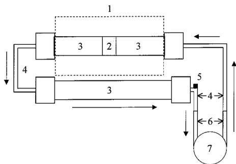
FIGURE 1. Experimental set-up. 1—temperature controlled chamber with four UV light sources; 2—illuminated section of glass tube (photocatalytic experiments only) randomly packed with eight catalyst-coated glass rings; 3—nonilluminated sections of glass tube (not packed with catalyst-coated glass rings); 4—stainless steel tubing; 5—sampling port (septum); 6—Viton pump tubing; 7—peristaltic pump.
