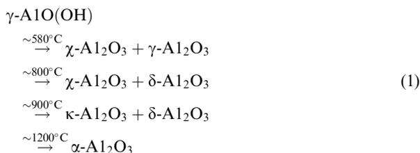
With the phase transformation sequences shown in Eq. (1), it is then possible to apply the phase analysis to estimate the temperature variation within the PECS powder compact.
