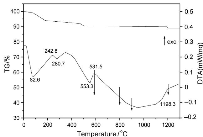
Fig. 1. Thermogravimetric analysis (TGA) and differential thermal analysis (DTA) curves of the aluminum hydroxide powder.
