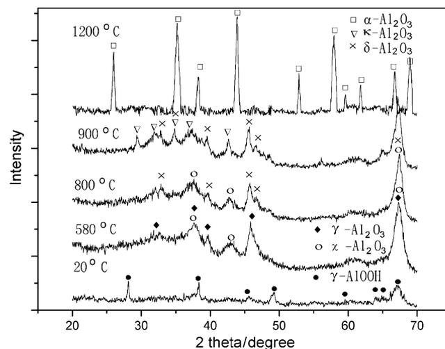
Fig. 2. X-ray diffractometry patterns for the aluminum hydroxide powder compacts after conventional heat treatment at various temperatures.
