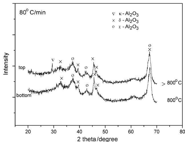
**Fig. 4.** X-ray diffractometry patterns for the aluminum hydroxide powder compacts after pulse electric current sintering at 900°C for 1 min at a heating rate of 80°C/min. A carbon paper separator is used.
