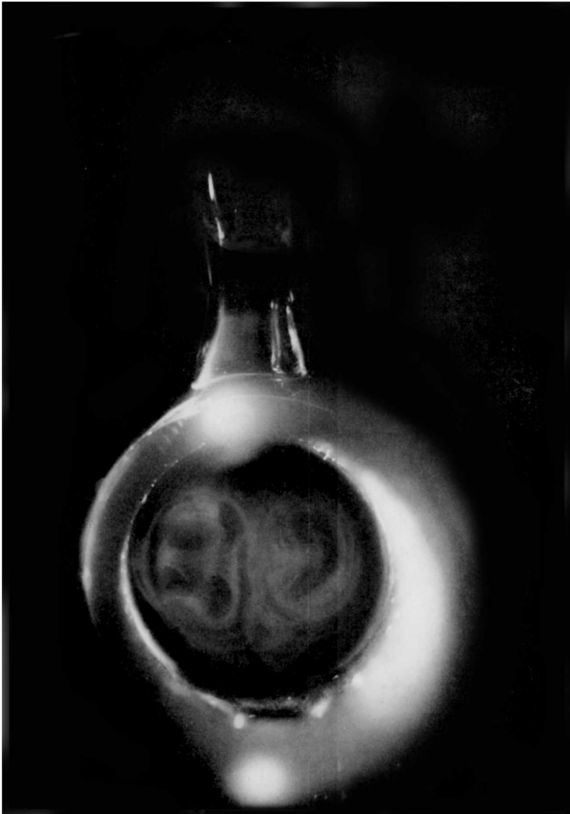
FIG. 6.—Gas-phase nucleation of carbonaceous solid from radiolysis of CO.
