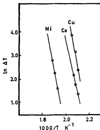
**Fig. 3** Plots constructed from the DTA curves of nitrate-complexes
