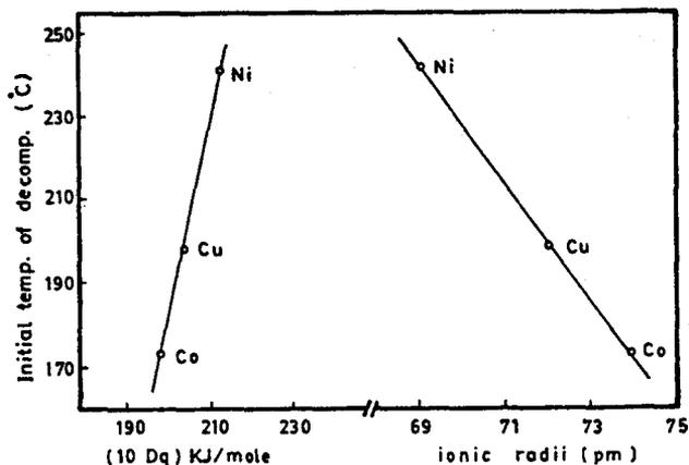
Fig. 4 A plot of ionic radii and crystal field splitting energy with the initial temperature of decomposition of nitrate-complexes
