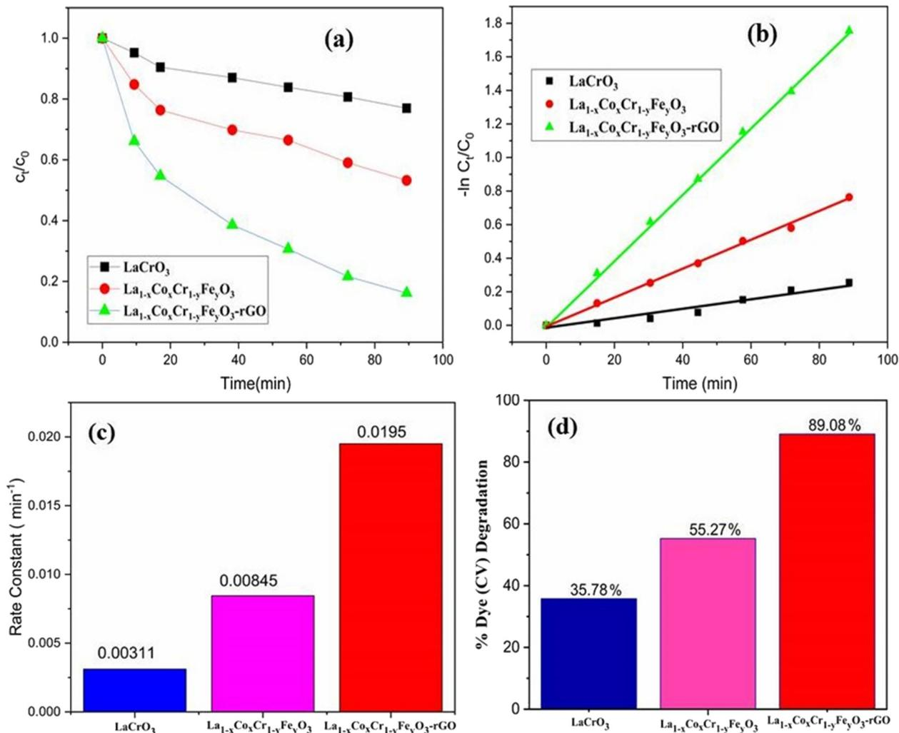
**Fig. 8.** Degradation curves profiles of CV dye over pristine  $\text{LaCrO}_3$ ,  $\text{La}_{1-x}\text{Co}_x\text{Cr}_{1-y}\text{Fe}_y\text{O}_3$  and  $\text{La}_{1-x}\text{Co}_x\text{Cr}_{1-y}\text{Fe}_y\text{O}_3/\text{r-GO}$ . (a) The degradation-rate, (b) Linear-kinetic, (c) Rate-constant and (d) percentage degradation of dye.
