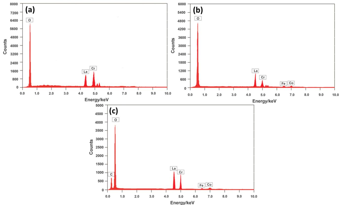
**Fig. 3.** EDX spectra, (a) pristine  $\text{LaCrO}_3$  NPs, (b) doped  $\text{La}_{1-x}\text{Co}_x\text{Cr}_{1-y}\text{Fe}_y\text{O}_3$  NPs and (c)  $\text{La}_{1-x}\text{Co}_x\text{Cr}_{1-y}\text{Fe}_y\text{O}_3/\text{r-GO}$  nanocomposite.
