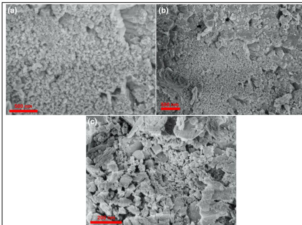
Fig. 2. SEM images, (a) pristine LaCrO<sub>3</sub> NPs, (b) doped La<sub>1-x</sub>Co<sub>x</sub>Cr<sub>1-y</sub>F<sub>y</sub>O<sub>3</sub> NPs and (c) La<sub>1-x</sub>Co<sub>x</sub>Cr<sub>1-y</sub>F<sub>y</sub>O<sub>3</sub>/r-GO nanocomposite.
