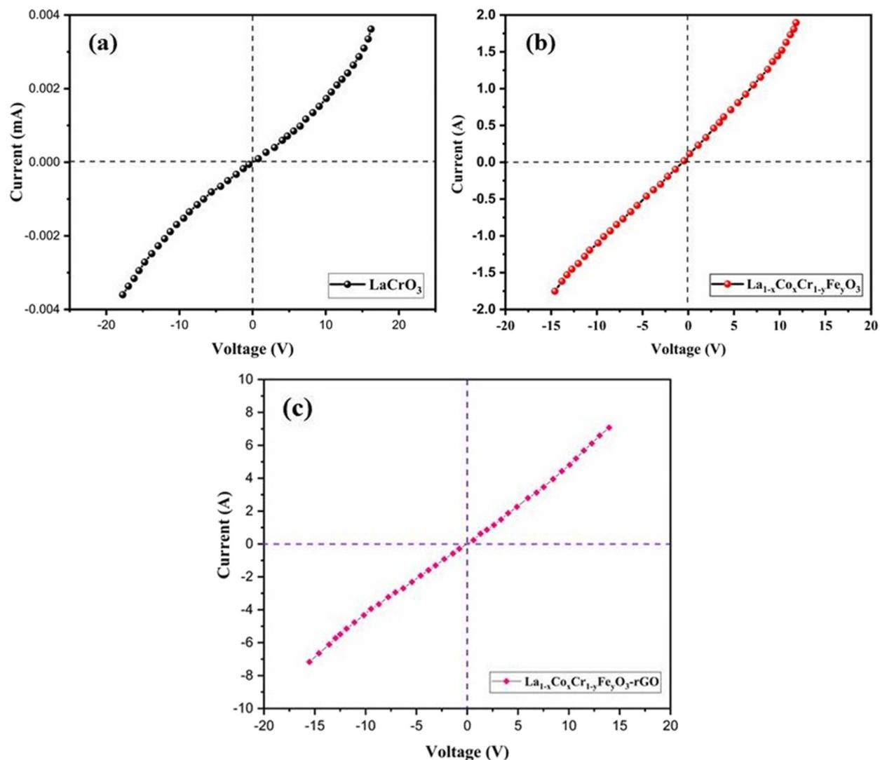
**Fig. 6.** I-V profiles of LaCrO<sub>3</sub>, (b) La<sub>1-x</sub>Co<sub>x</sub>Cr<sub>1-y</sub>Fe<sub>y</sub>O<sub>3</sub> NPs (c) La<sub>1-x</sub>Co<sub>x</sub>Cr<sub>1-y</sub>Fe<sub>y</sub>O<sub>3</sub>/r-GO nanocomposite.
