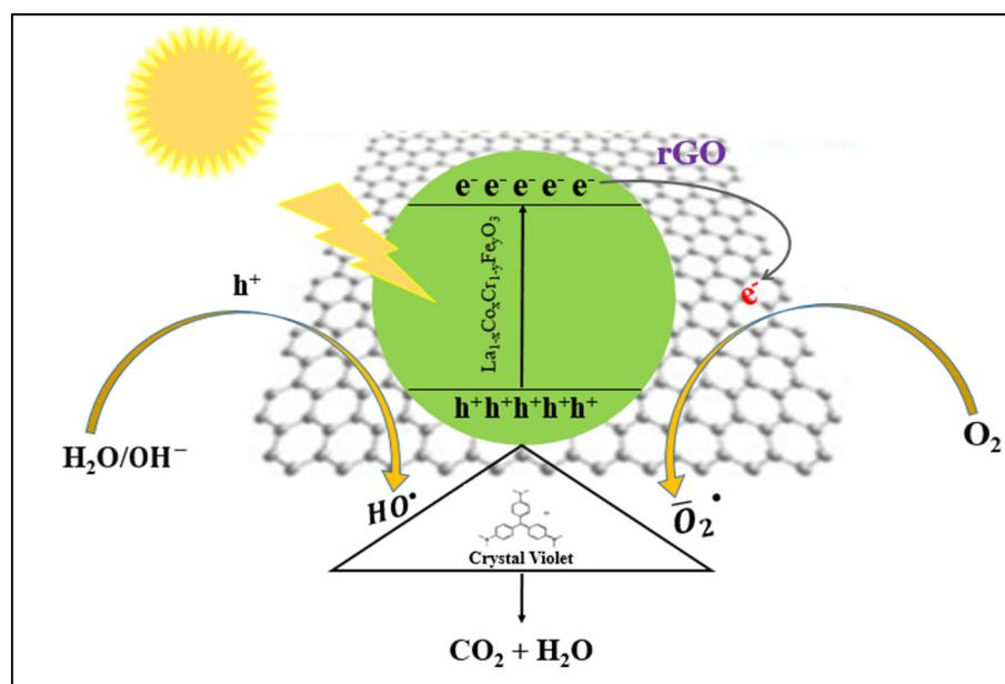
**Fig. 10.** Photocatalytic proposed mechanism for dye degradation over  $\text{La}_{1-x}\text{Co}_x\text{Cr}_{1-y}\text{Fe}_y\text{O}_3/\text{r-GO}$  photocatalyst.
