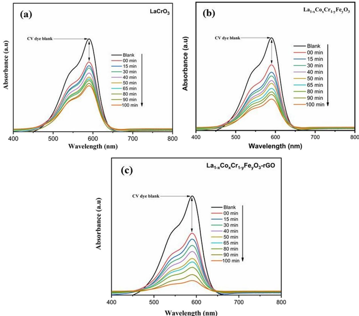
**Fig. 7.** Absorption spectra of CV dye photo-degradation over, (a) pristine LaCrO<sub>3</sub> (b) doped La<sub>1-x</sub>Co<sub>x</sub>Cr<sub>1-y</sub>Fe<sub>y</sub>O<sub>3</sub> and (c) La<sub>1-x</sub>Co<sub>x</sub>Cr<sub>1-y</sub>Fe<sub>y</sub>O<sub>3</sub>/r-GO nanocomposite.
