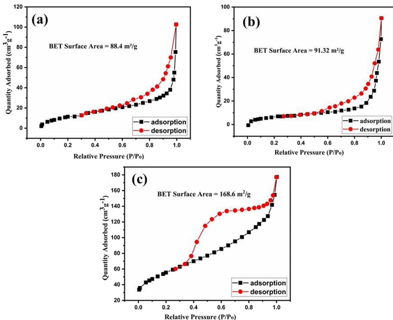
**Fig. 5.** Nitrogen physisorption isotherms, (a) pristine  $\text{LaCrO}_3$ , (b)  $\text{La}_{1-x}\text{Co}_x\text{Cr}_{1-y}\text{Fe}_y\text{O}_3$  NPs (c)  $\text{La}_{1-x}\text{Co}_x\text{Cr}_{1-y}\text{Fe}_y\text{O}_3/\text{r-GO}$  nanocomposite.
