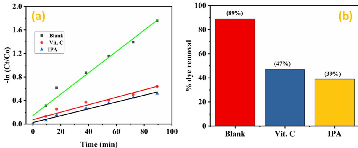
**Fig. 9.** (a) Photocatalytic degradation of CV over  $\text{La}_{1-x}\text{Co}_x\text{Cr}_{1-y}\text{Fe}_y\text{O}_3/\text{r-GO}$  photo-catalyst alone and with different scavengers and (b) dye removal percentages in the presence of scavengers.
