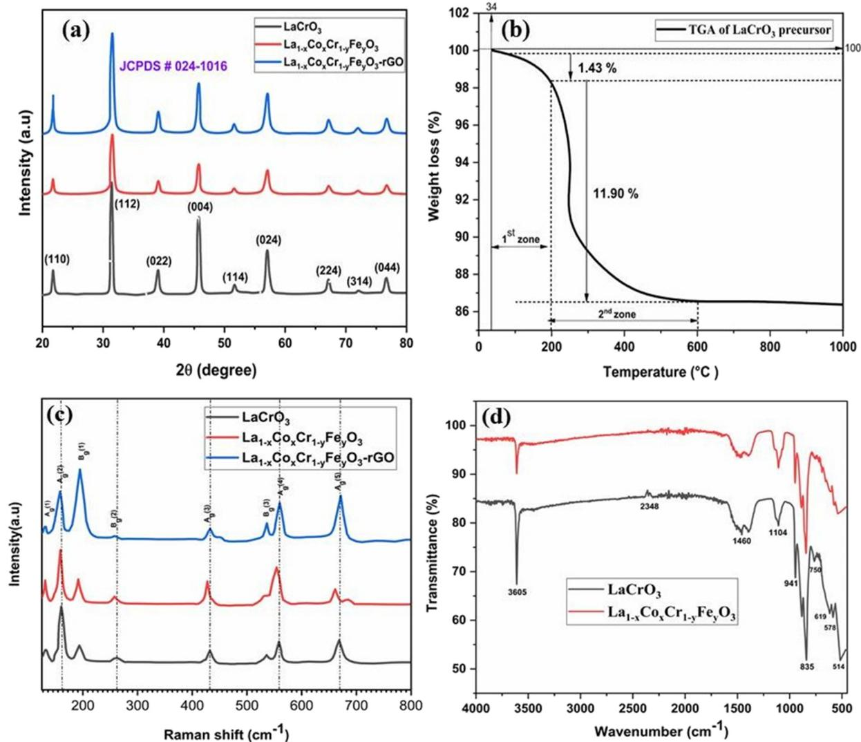
**Fig. 4.** (a) XRD pattern of fabricated NPs, (b) TGA curve of pristine  $\text{LaCrO}_3$  NPs, (c) Raman spectra, (d) FTIR spectra of pristine  $\text{LaCrO}_3$  and doped  $\text{La}_{1-x}\text{Co}_x\text{Cr}_{1-y}\text{Fe}_y\text{O}_3$  NPs.
