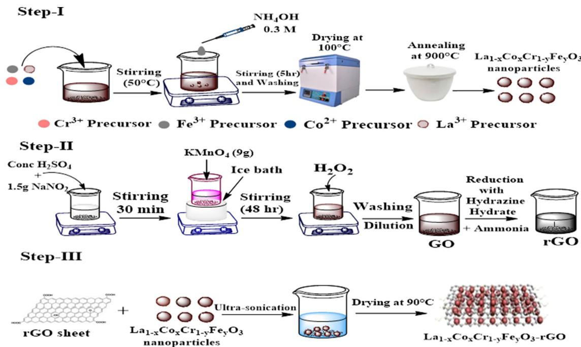
Fig. 1. Schematic flow sheet diagram for the formation of La<sub>1-x</sub>Co<sub>x</sub>Cr<sub>1-y</sub>F<sub>y</sub>O<sub>3</sub> NPs (Step 1), r-GO (Step II), and their nanocomposite (Step III).
