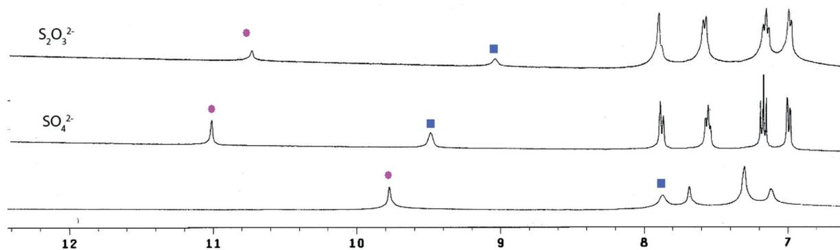
**Fig. 6** Partial  $^1\text{H}$  NMR spectra (400 MHz,  $\text{DMSO-d}_6$ ) of **L** and maximum observable shifts of thiourea –NH resonances upon the addition of excess (5 equiv.)  $\text{SO}_4^{2-}$  and  $\text{S}_2\text{O}_3^{2-}$  anions.
