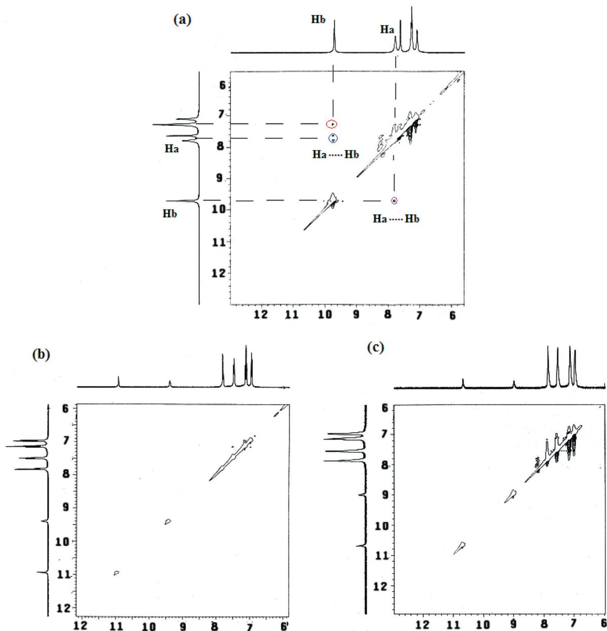
**Fig. 8** 2D NOESY NMR experiments of: (a) free receptor **L**; (b) **L** in presence of 1 equiv. of sulfate anion; and (c) **L** in presence of 1 equiv. of thio-sulfate anion. All the spectra are taken in DMSO-*d*<sub>6</sub> at 298K.
