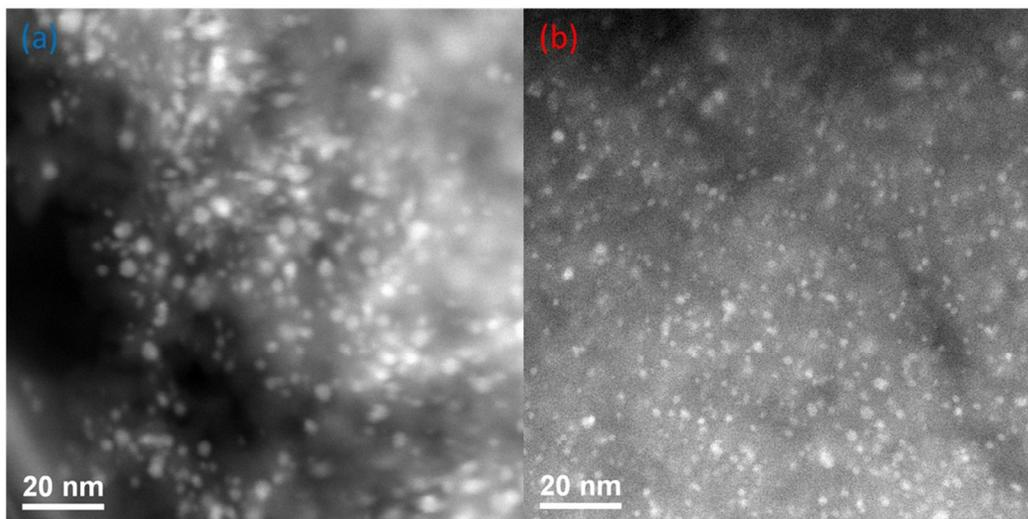
**Figure 4.** STEM images of (a) Pt/SiO<sub>2</sub>, (b) Pt/H-ZSM-5 catalysts.
