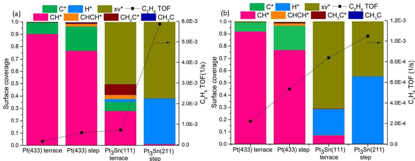
**Figure 10:** Surface coverages and ethylene TOF values of the studied surfaces predicted by the microkinetic model (a) no co-feeding conditions (b) 5% H<sub>2</sub> co-feeding with methane. (Experimental conditions same as Figure 1 and Figure 2) Left axis shows surface coverage of the indicated species, right axis shows the ethylene TOF values.
