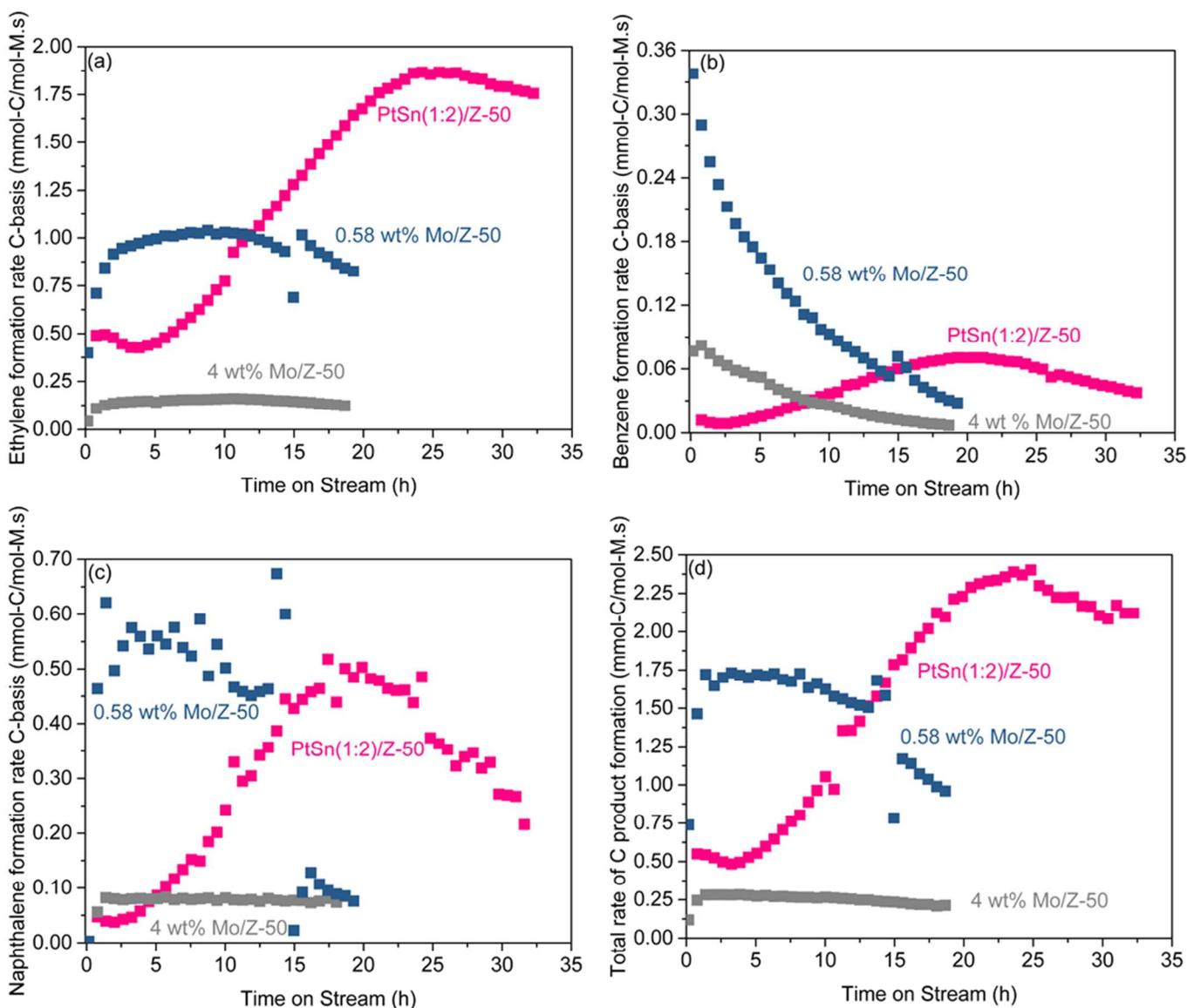
**Figure 8.** Rate of carbon product formation from (a) ethylene (b) benzene (c) naphthalene on the 0.58 wt% Pt-Sn(1:2)/Z-50, 0.58 wt% Mo/Z-50 and 4 wt% Mo/Z-50 catalysts. (d) Total rate of carbon product formation on each catalyst. *Conditions:* CH<sub>4</sub> flowrate = 10.5 cm<sup>3</sup>(STP)/min, T = 973 K, catalyst mass = 0.25 g.
