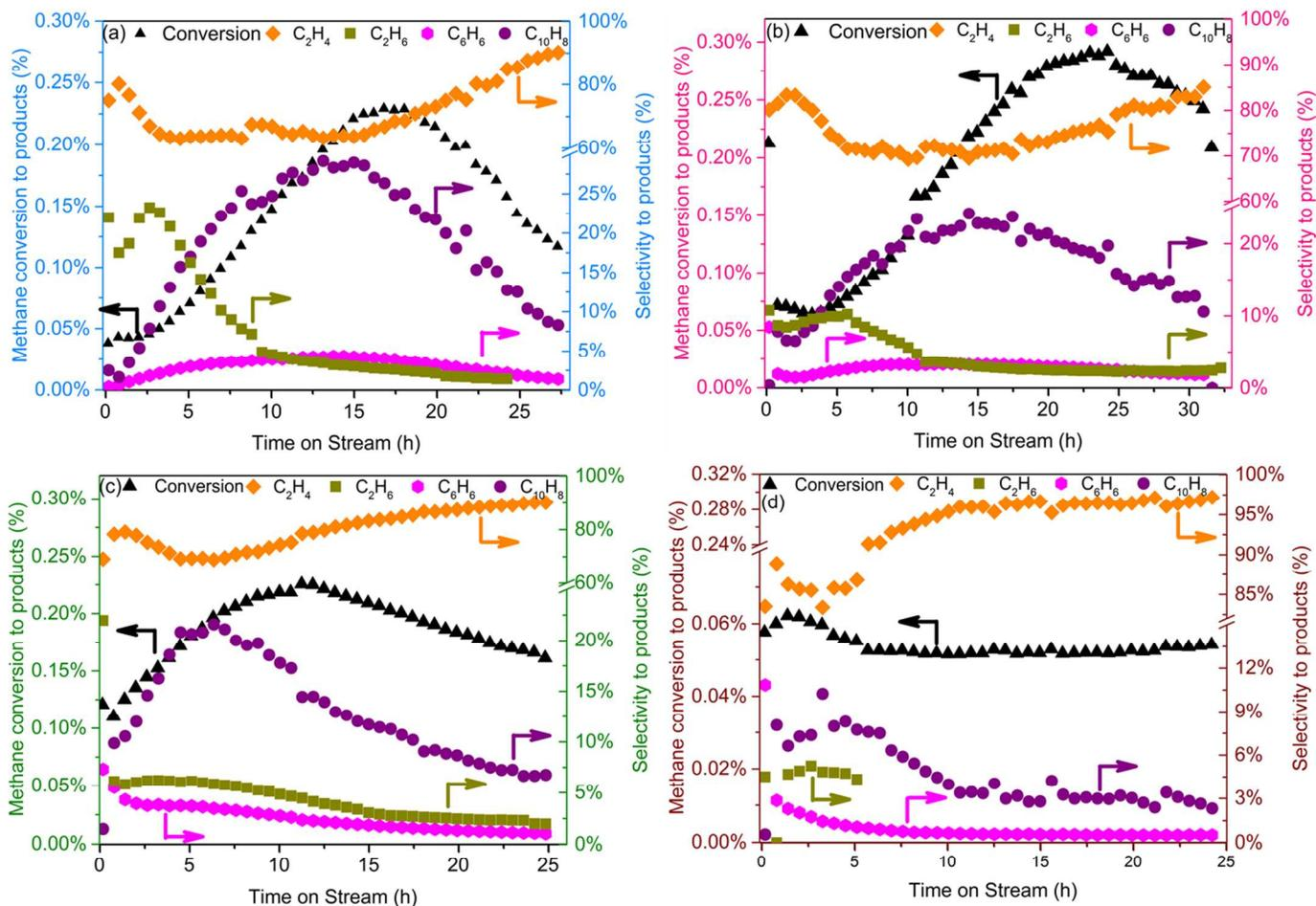
**Figure 7.** Effect of support acidity on methane conversion to detectable products and selectivities of (a) PtSn(1:2)/Z-23, (b) PtSn(1:2)/Z-50 (c) PtSn(1:2)/Z-80 and (d) PtSn(1:2)/Z-280. Conditions: CH<sub>4</sub> flowrate = 10.5 cm<sup>3</sup>(STP)/min, T = 973 K, catalyst mass = 0.25 g.
