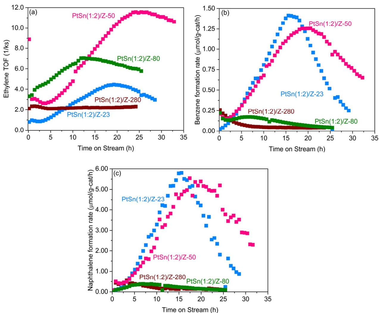
**Figure 6.** Effect of support acidity on (a) ethylene TOF (b) benzene formation rate and (c) naphthalene formation rate of zeolite-supported catalysts. *Conditions:*  $\text{CH}_4$  flowrate = 10.5  $\text{cm}^3(\text{STP})/\text{min}$ ,  $T = 973 \text{ K}$ , catalyst mass = 0.25 g.
