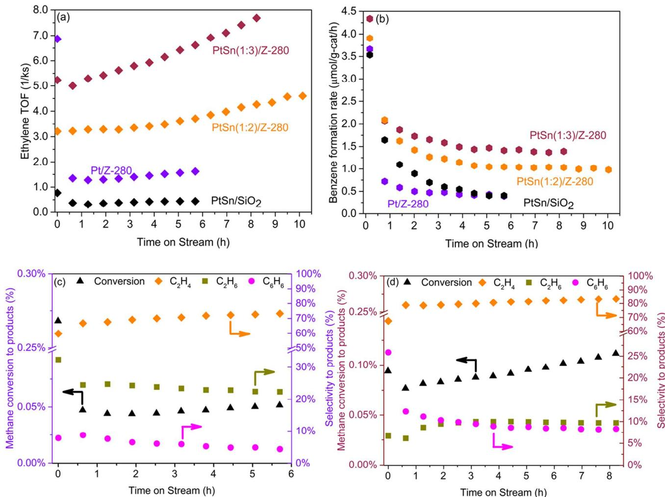
**Figure 3.** Effect of Sn addition to Pt/Z-280. (a) Ethylene TOF (b) benzene formation rate per mass of catalyst over Pt/Z-280 and PtSn/Z-280, methane conversion to detectable products and selectivities excluding coke for (c) Pt/Z-280 and (d) PtSn(1:3)/Z-280. Ethylene TOF and benzene formation rate over PtSn/SiO<sub>2</sub> (overall atomic ratio of Pt/Sn equal to 3:1) are given for comparison. *Conditions:* CH<sub>4</sub> flowrate = 42 cm<sup>3</sup>(STP)/min, T = 973 K, catalyst mass = 1 g.
