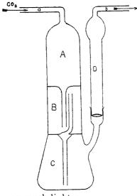
partments B and C contain as much of the solution as would completely fill A, which is about thirty-five to forty grams of a 2; 3 solution. D, which is fastened to the bulb by means of a ground-glass joint, contains solid potassium hydroxide, or soda-lime, supported by a plug of glass-wool. The liquids in B and C can be easily mixed when desired, by applying suction at a. The bulb, when filled and ready for use, weighs from sixty-five to seventy grams, and undoubtedly can be made
