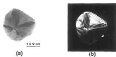
Figure 5. Decahedral Ag particle (a) formed in 50 mM CsClO 4 + 1 mM AgClO 4 solution at 0 V for 60 s and its dark field image (b).
