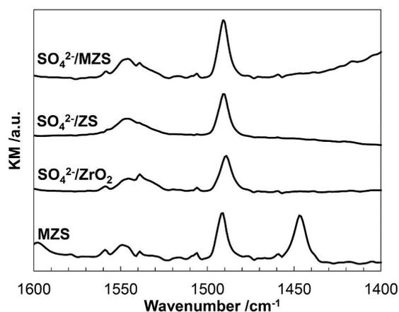
Fig. 5. DRIFT difference spectra before and after pyridine adsorption.
