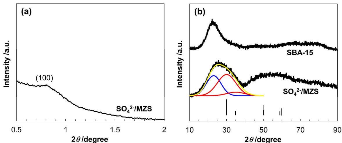
Fig. 2. SAXS (a) and XRD (b) patterns of prepared samples. Vertical lines in (b) indicate position of major diffraction peaks for tetragonal zirconia. Color lines show deconvolution.
