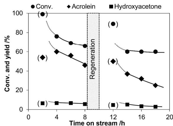
Fig. 6. Effect of time on stream and regeneration on conversion of glycerol over  $\text{SO}_4^{2-}/\text{MZS}$ .
