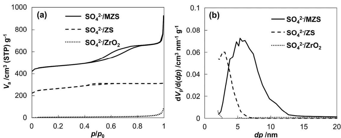
Fig. 1. N<sub>2</sub> adsorption isotherms (a) (baseline shifted) and BJH plots (b) of sulfated zirconia derivatives.
