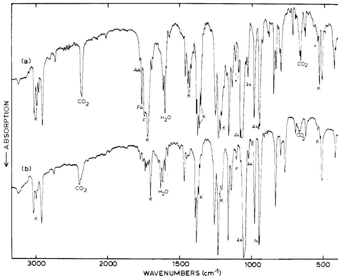
**Figure 5.** Infrared spectra of the reaction product of methylpropene in Freon-13 solution evaporated from U-tube at  $-77$  to  $-10$  °C and codeposited with argon at 15 K: (a)  $^{16}\text{O}_3$ , (b)  $^{18}\text{O}_3$ . *r* denotes bands that remain on photolysis. *2a* denotes cross ozonide.
