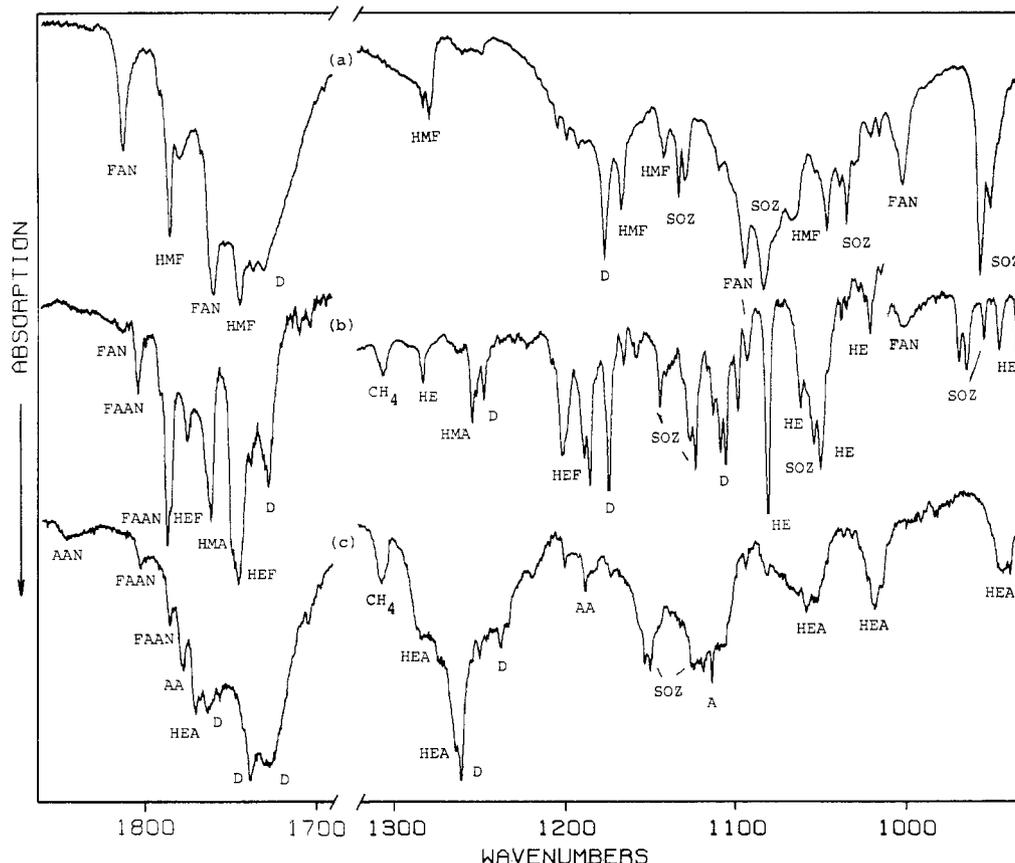
**Figure 3.** Infrared spectra of the matrix photolysis products of SOZ samples in 930–1320- and 1690–1860-cm<sup>-1</sup> spectral regions: (a) ethene-SOZ, (b) propene-SOZ, (c) 2-butene-SOZ.
