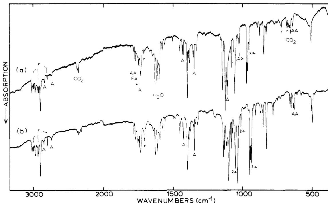
**Figure 2.** Infrared spectra of the product of the propene-ozone reaction in Freon-13 solution evaporated from U-tube at  $-77^{\circ}\text{C}$  and codeposited with argon at 15 K: (a)  $^{16}\text{O}_3$ , (b)  $^{18}\text{O}_3$ . 2a denotes ethene-SOZ cross ozonide; r denotes bands that remain on photolysis.
