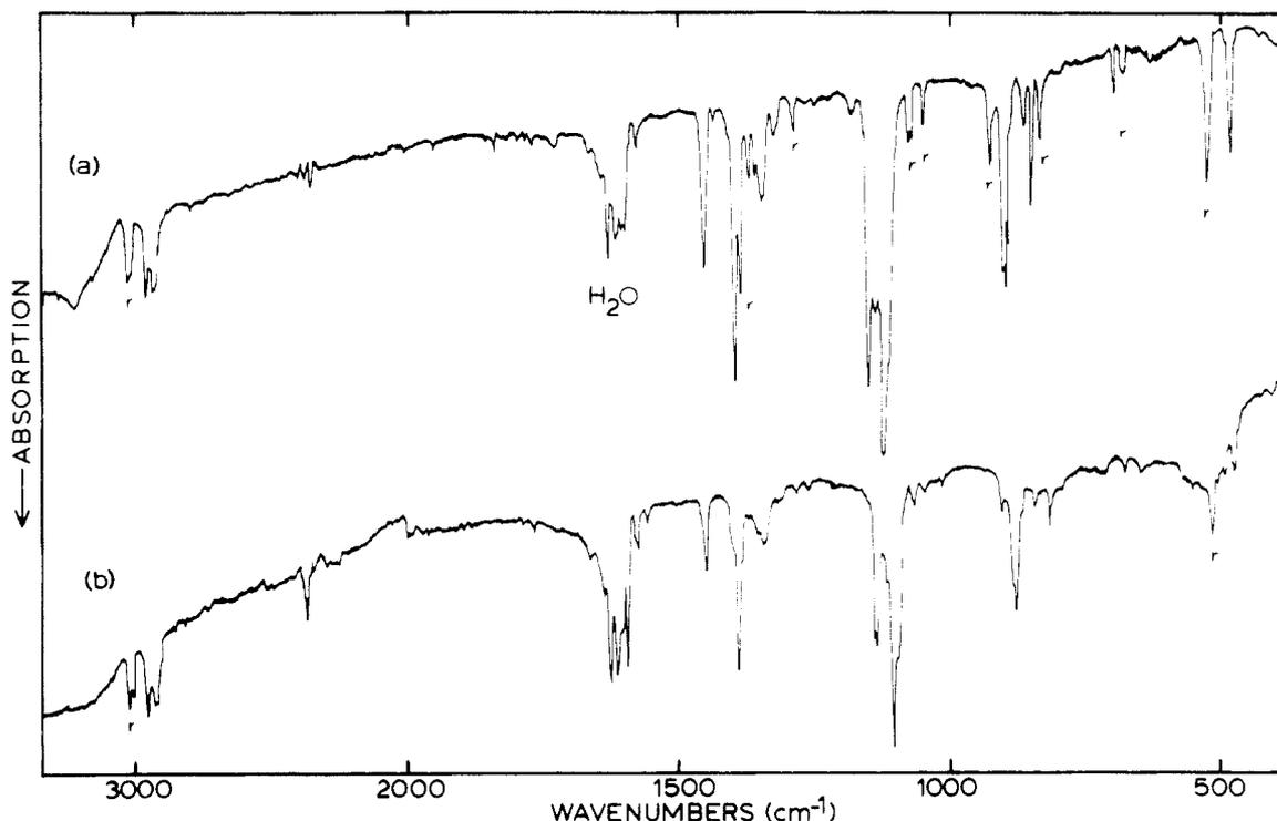
**Figure 4.** Infrared spectra of the reaction product of *trans*-2-butene and ozone in Freon-13 solution evaporated from U-tube at  $-25^{\circ}\text{C}$  and codeposited with argon at 15 K: (a)  $^{16}\text{O}_3$ , (b)  $^{18}\text{O}_3$ . r denotes bands that remain on photolysis.
