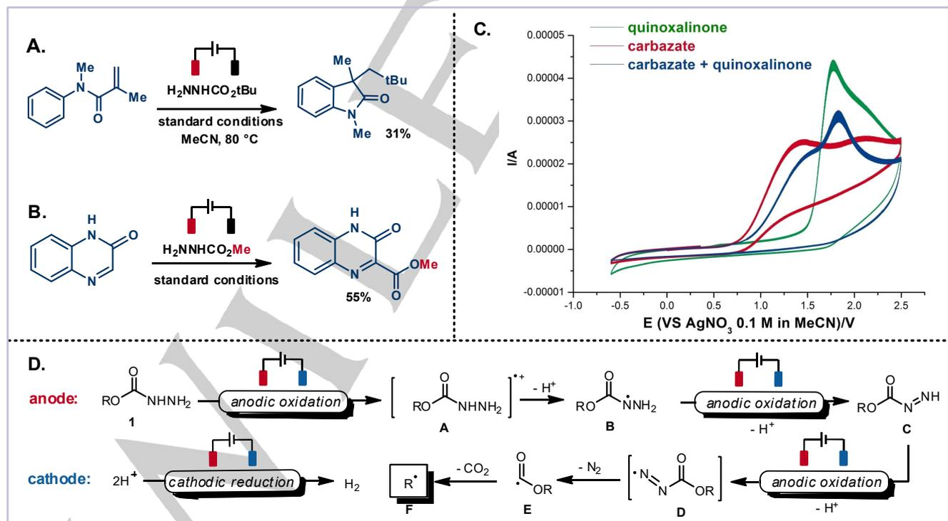
**Scheme 3.** Control experiments and reaction mechanism. A) Cyclic voltammetry of related compounds in 0.1 M n-Bu<sub>4</sub>NPF<sub>6</sub>/MeCN using glass carbon working electrode, Pt wire, and Ag/AgNO<sub>3</sub> (0.1 M in MeCN) as counter and reference electrode: 2-quinoxalione (5 mM, green); t-butyl carbazate (5 mM, red); 2-quinoxalione and t-butyl carbazate (5 mM, blue).
