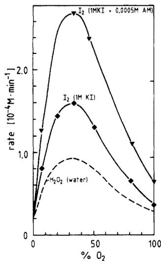
**Figure 3.** Irradiation of 0.1 M KI solutions (solid lines) under various mixtures of argon and oxygen. The dashed curve gives the  $\text{H}_2\text{O}_2$  yield from water (from Figure 1).
