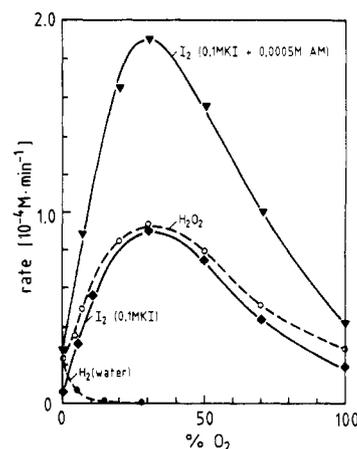
Figure 1. Irradiation of water (dashed lines) and of a 0.1 M KI solution (solid lines) under various mixtures of argon and oxygen (the composition of the gas mixture is given in volume percent of O<sub>2</sub>).
