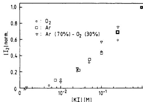
**Figure 4.**  $\text{I}_2$  yield as a function of iodide concentration in the irradiation under argon, oxygen, and argon (70%)–oxygen (30%). Yields are normalized for  $[\text{I}^-] = 1$  M.
