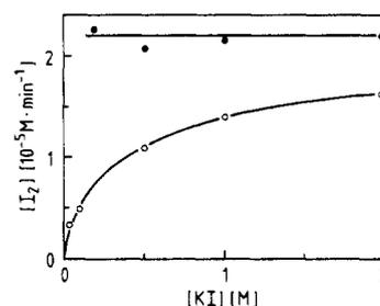
Figure 2. Yield of I<sub>2</sub> as a function of the KI concentration in the irradiation of solutions under argon in the absence (O) and presence (●) of 5 × 10<sup>-4</sup> M ammonium molybdate. The rate of H<sub>2</sub>O<sub>2</sub> formation in pure water was 2.2 × 10<sup>-5</sup> M min<sup>-1</sup>.
