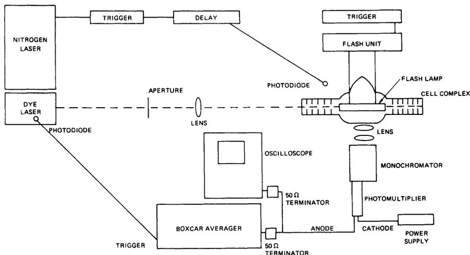
**Fig. 1.** The experimental arrangement for the CN studies using the flash photolysis/laser-induced fluorescence technique.
