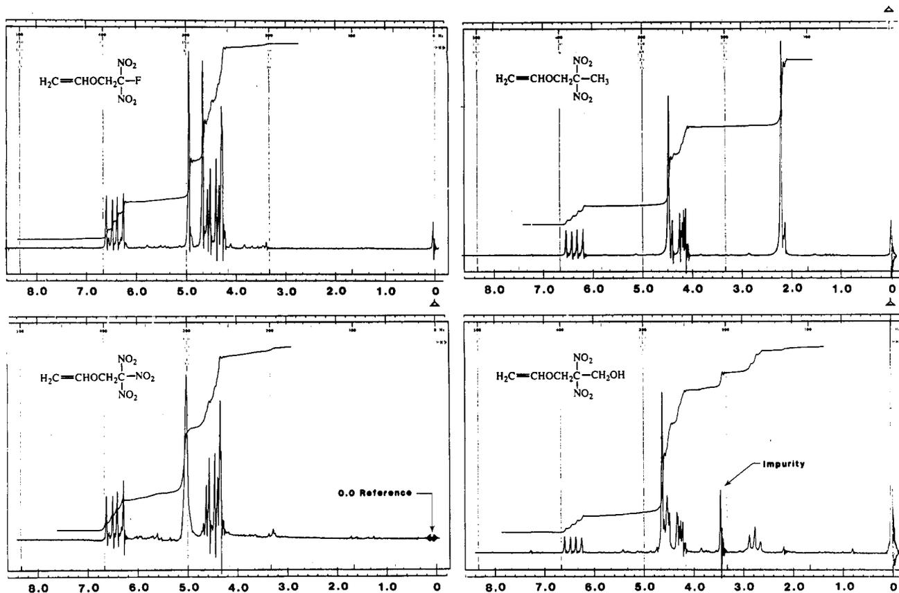
Figure 1. NMR (60-Hz) spectra of vinyl ether products 5-8.
