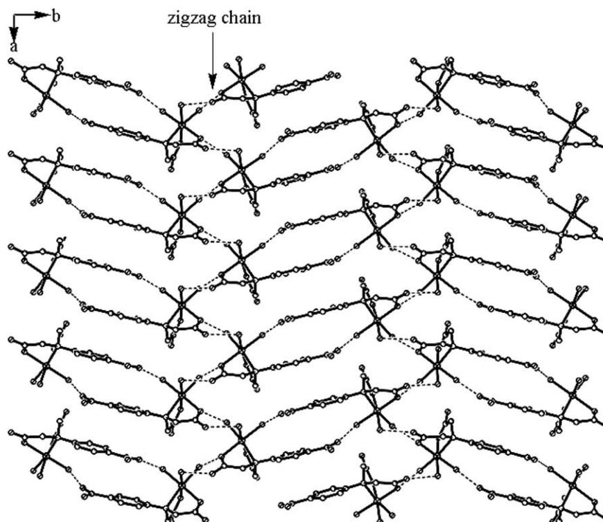
Fig. 2. Two-dimensional supramolecular network in **1** as viewed down the *c* axis, showing the double hydrogen-bond-linked zigzag-shape chains, the dotted lines represent hydrogen bonds.
