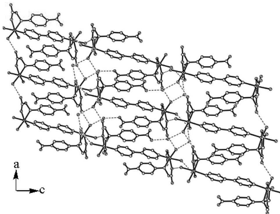
Fig. 5. View of two-dimensional joint-ladder like supramolecular network of **2** down the *b* axis, showing the double hydrogen-bond-linked ladder-shape chains, the dotted lines represent hydrogen bonds.
