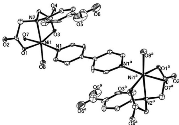
Fig. 4. Perspective view of the coordination environment of the nickel atoms in compound **2**, showing Z-shape dimer; thermal ellipsoids are drawn at the 50% probability level; all hydrogen atoms and uncoordinated water molecules are omitted for clarity; Symmetry code:  $a = -x, -y, -z$ .
