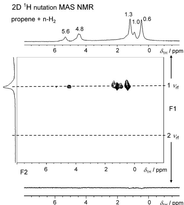
**Figure 3.** In situ 2D  $^1\text{H}$  nutation MAS NMR spectrum (middle) recorded during hydrogenation of propene with  $n\text{-H}_2$  on 0.9Pt/silica at 373 K and slices of this spectrum at the nutation frequencies of  $1\nu_{\text{rf}}$  (top) and  $2\nu_{\text{rf}}$  (bottom).
