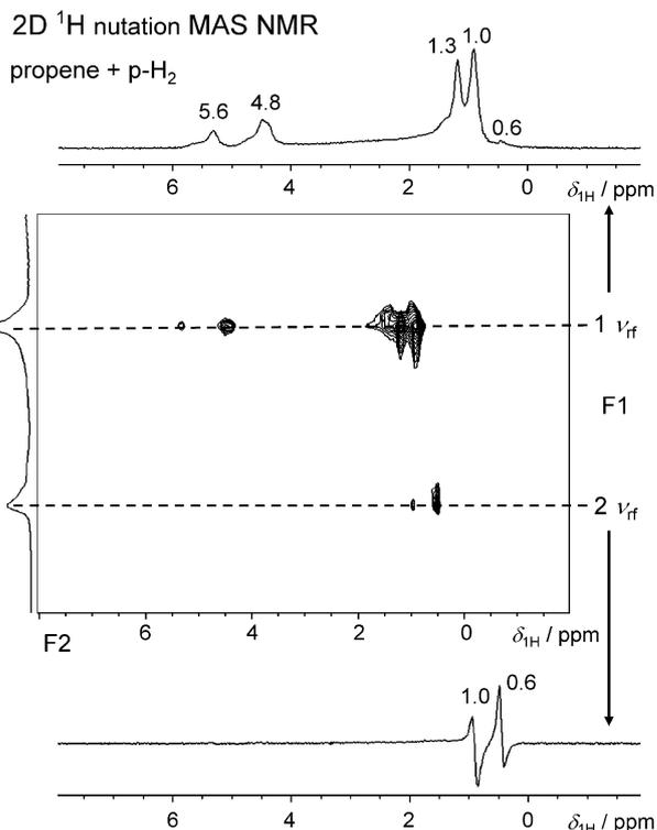
**Figure 4.** In situ 2D  $^1\text{H}$  nutation MAS NMR spectrum (middle) recorded during hydrogenation of propene with  $p\text{-H}_2$  on 0.9Pt/silica at 373 K and slices of this spectrum at the nutation frequencies of  $1\nu_{\text{rf}}$  (top) and  $2\nu_{\text{rf}}$  (bottom).
