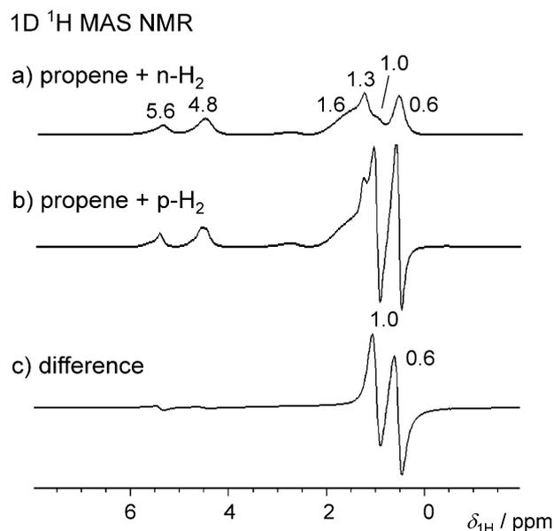
**Figure 2.** In situ 1D  $^1\text{H}$  MAS NMR spectra recorded during the hydrogenation of propene with n- $\text{H}_2$  (top) and p- $\text{H}_2$  (middle) on 0.9Pt/silica under continuous-flow conditions at 373 K. The bottom spectrum is the difference of the spectra recorded during hydrogenation with n- $\text{H}_2$  and p- $\text{H}_2$ .
