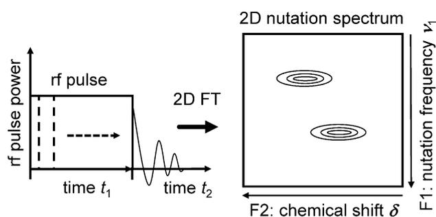
**Figure 1.** Scheme of the 2D nutation NMR experiment and the nutation spectrum obtained upon 2D Fourier transformation (2D FT) for the time domains  $t_1$  (incremented pulse length) and  $t_2$  (induction decays).
