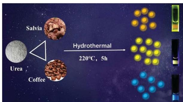
Fig. 1 Diagram for the fabrication of concentration-dependent multicolor fluorescent CDs.
