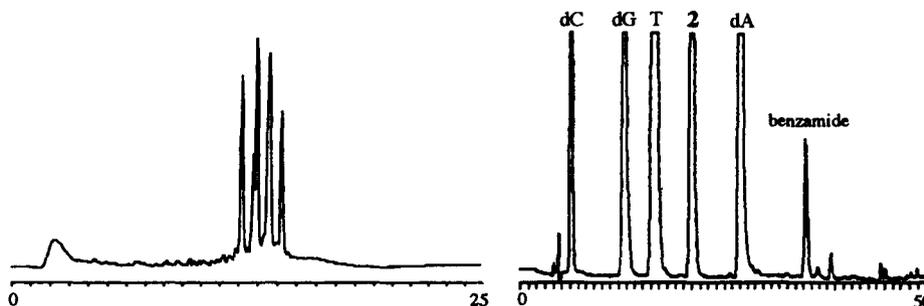
Figure 1. Anion-exchange HPLC (left) and RP HPLC of enzymatic digest (right) of 18mer 5' TCA CAG TCT GAT CTC GAT 3' made with 0.1M iodine oxidation reagent
