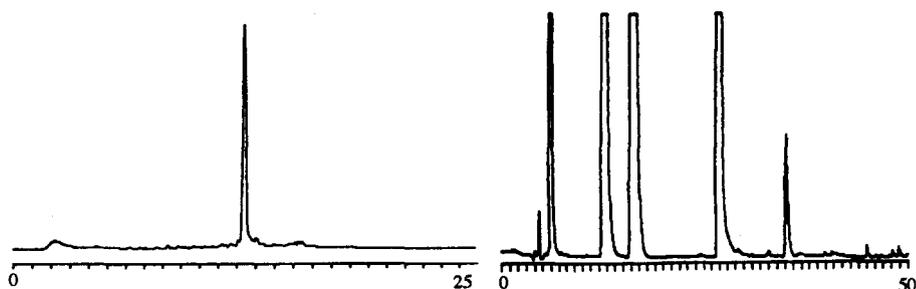
Figure 3. Anion-exchange HPLC (left) and RP HPLC of enzymatic digest (right) of 18mer 5' TCA CAG TCT GAT CTC GAT 3' made with 0.02M iodine oxidation reagent
