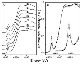
Figure 3. Ti K-edge XANES spectra of (A) all analyzed samples as synthesized and (B) details of XANES spectra evolution on 3a as prepared, in air (-●-); in an Ar atmosphere after dehydration in Ar, 2 h at 393 K (-); and in an Ar atmosphere after dehydration in Ar, 2 h at 523 K (-0-). The inset amplifies the corresponding pre-edge region.
