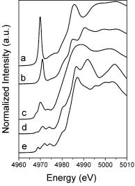
Figure 2. Ti K-XANES spectra of reference Ti-compounds at ambient temperature in air: (a) 4-fold coordinate [4]Ti in Ba<sub>2</sub>TiO<sub>4</sub>; (b) [5]Ti in Fresnoite; (c) [5]Ti in nanostructured anatase (average crystal size <6 nm),59 (d) [6]Ti in rutile, and (e) [6]Ti in anatase.
