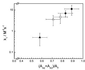
Figure 7. Epoxidation rate constants per Ti as a function of the relative area of peaks A2 + A3 for Ti-containing materials 3a-393 (●), 3a-823 (○), 3b-393 (■), 3c-393 (▲), and 3c-823 (△). Error bars are estimated from confidence of fitting procedures. Use of the A2 + A3 relative peak area rather than the total pre-edge feature height predicts a monotonic relationship between catalyst reactivity and Ti K-edge XANES for all calixarene-containing and calcined Ti-SiO<sub>2</sub> materials.
