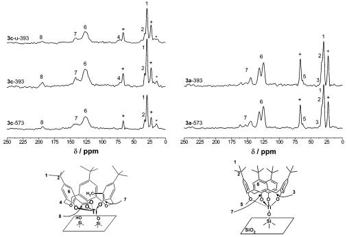
Figure 1. Solid-state <sup>13</sup>C CP/MAS NMR spectra of 3a and 3c. Resonances are labeled as in the accompanying structures. (\*) indicates spinning sideband and (+) indicates resonances due to surface isopropoxy groups, the latter of which is emblematic of covalent surface grafting of the Ti complex. The resonance at ~190 ppm is indicative of a carbonyl group, whose intensity is extremely sensitive to catalyst pretreatment, presumably due to the long relaxation time of this group.
