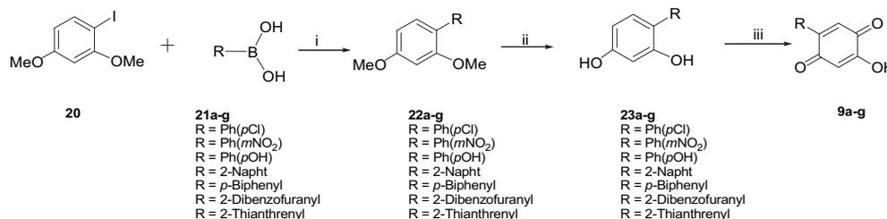
**Scheme 5.** Reagents and conditions: (i) K<sub>2</sub>CO<sub>3</sub>, PdCl<sub>2</sub>(dppf), Ethanol, MW, 25 min; (ii) BBr<sub>3</sub>, CH<sub>2</sub>Cl<sub>2</sub>, –15 °C to rt, 18 h; (iii) NO(KSO<sub>3</sub>)<sub>2</sub>, EtOAc–H<sub>2</sub>O, Na<sub>2</sub>HPO<sub>4</sub>, 0 °C to rt, 20 h.
