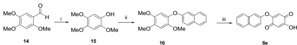
**Scheme 3.** Reagents and conditions: (i)  $H_2O_2$ ,  $H_2SO_4$ , MeOH, rt, 2.5 h; (ii) 2-naphthyl boronic acid,  $Cu(OAc)_2$ , pyridine,  $CH_2Cl_2$ , rt, 48 h; (iii) CAN,  $CH_3CN$ , rt, 1 h.
