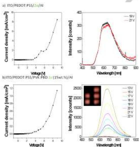
Figure 5. Current density-voltage characteristics and electroluminescence spectra of OLED for increasing and decreasing voltage registered for devices with (a) ITO/PEDOT:PSS/2a/Al and (b) ITO/PEDOT:PSS/PVK:PBD:1c/Al structure.
