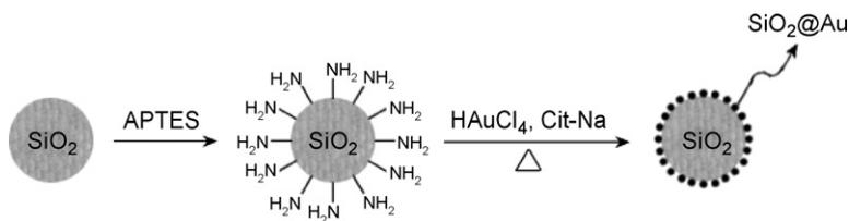
Fig. 2. Schematic illustration of the deposition of Au NPs onto silica microspheres II.
