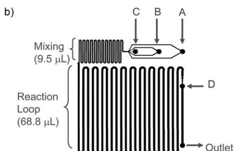
**Figure 1.** a) Microreactor setup. b) Schematic representation of the microreactor showing the three inlets (acid fluoride (A), amino acid benzyl ester (B) and *N*-methylmorpholine (NMM; C)), the quench port (TFA and the internal standard (D)), the outlet, and the dimensions of the channels (total prequench reactor volume = 78.3  $\mu\text{L}$ ).
