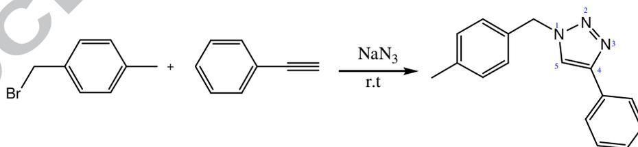
**Scheme 4:** Cycloaddition reaction of 4-methylbenzyl bromide and phenylacetylene with NaN<sub>3</sub> at room temperature.
