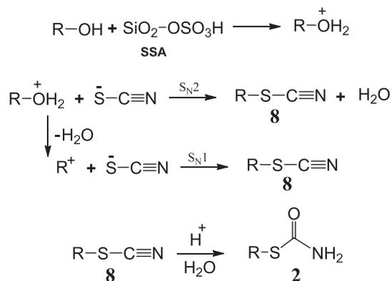
Scheme 5. Suggested mechanism of synthesis of *S*-alkylthiocarbamates **2** via thiocyanation of alcohols.
