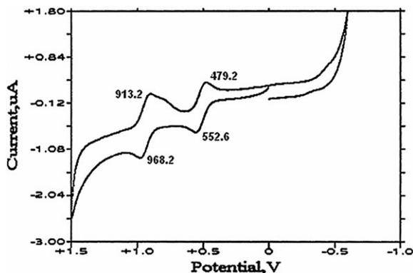
Fig. 1 Cyclic voltammogram (CV) for **10a** (DCM, electrolyte TBAPF<sub>6</sub>; working electrode: Pt; reference electrode: Ag/AgCl; 80 mV s<sup>-1</sup> (for CV of **10b** and **10c**, see Fig. S1 and S2, ESI<sup>†</sup>).
