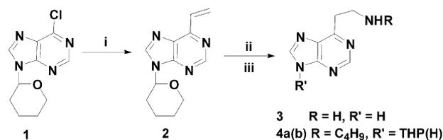
**Scheme 1.** Regents and conditions: (i) (Ph<sub>3</sub>P)<sub>2</sub>PdCl<sub>2</sub>, tributylvinyltin, DCE, reflux; (ii) NH<sub>3</sub>/CH<sub>3</sub>OH or n-butylamine/DCM, rt; (iii) DCM/CH<sub>3</sub>OH, 1M HCl, rt.
