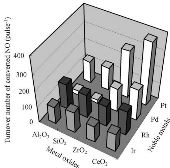
Fig. 6. Turnover number of converted NO per gas pulse on a metal atom of Pt, Pd, Rh and Ir catalysts, individually supported on Al<sub>2</sub>O<sub>3</sub>, SiO<sub>2</sub>, ZrO<sub>2</sub> and CeO<sub>2</sub> at 400 °C.
