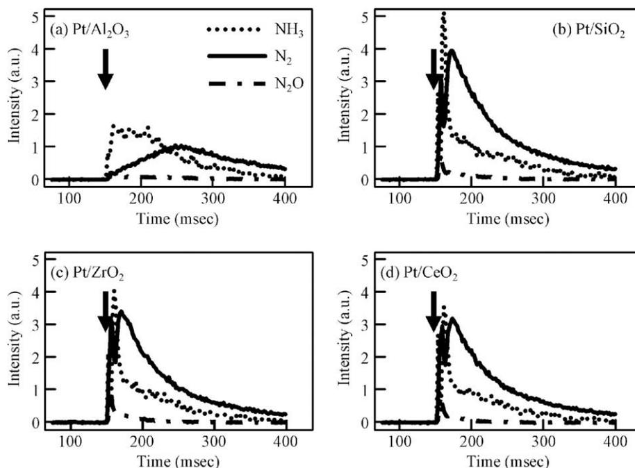
Fig. 1. Transient  $\text{NH}_3$ ,  $\text{N}_2$  and  $\text{N}_2\text{O}$  production from Pt catalysts supported on (a)  $\text{Al}_2\text{O}_3$ , (b)  $\text{SiO}_2$ , (c)  $\text{ZrO}_2$  and (d)  $\text{CeO}_2$  at 500 °C triggered by simultaneous injection of  $\text{H}_2$  and NO pulses as indicated by thick arrow.
