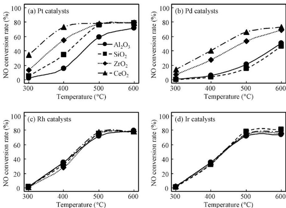
**Fig. 3.** Temperature dependence of the NO conversion rates over (a) Pt, (b) Pd, (c) Rh and (d) Ir catalysts.
