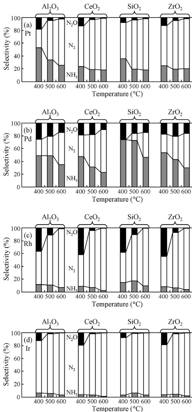
Fig. 4. Temperature dependence of the selectivity for  $\text{NH}_3$ ,  $\text{N}_2$  and  $\text{N}_2\text{O}$  over (a) Pt, (b) Pd, (c) Rh and (d) Ir catalysts.
