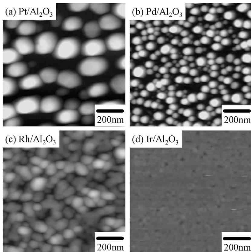
Fig. 5. AFM images of surface topography of (a) Pt, (b) Pd, (c) Rh and (d) Ir catalysts supported on Al<sub>2</sub>O<sub>3</sub>.
