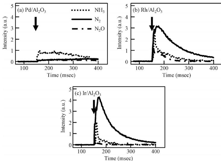
**Fig. 2.** Transient  $\text{NH}_3$ ,  $\text{N}_2$  and  $\text{N}_2\text{O}$  production from (a) Pd, (b) Rh and (c) Ir catalysts supported on  $\text{Al}_2\text{O}_3$  at  $500^\circ\text{C}$  triggered by simultaneous injection of  $\text{H}_2$  and  $\text{NO}$  pulses as indicated by thick arrow.
