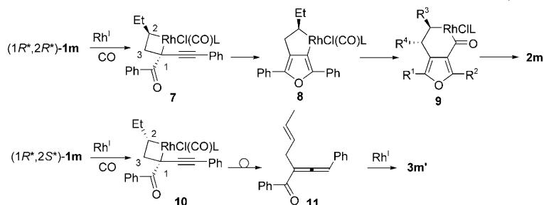
Scheme 2. Plausible mechanism of this carbonylation reaction.
